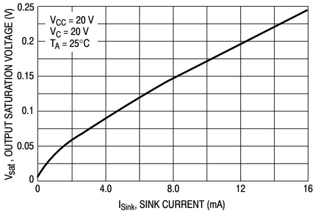
Figure 12. Fault Output Saturation Voltage versus Sink Current
