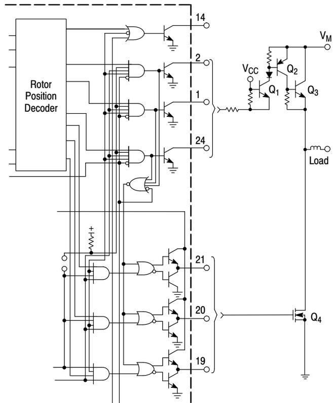
Transistor Q<sub>1</sub> is a common base stage used to level shift from V<sub>CC</sub> to the high motor voltage, V<sub>M</sub>. The collector diode is required if V<sub>CC</sub> is present while V<sub>M</sub> is low.
