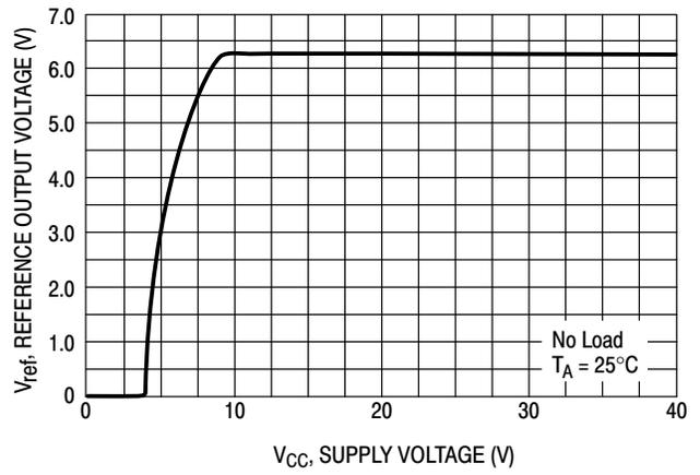
Figure 8. Reference Output Voltage versus Supply Voltage
