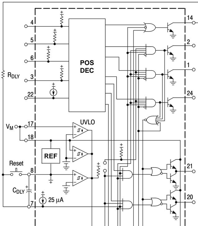
$$t_{DLY} \approx R_{DLY} C_{DLY} \ln \left( \frac{V_{ref} - (I_{IL\ enable} R_{DLY})}{V_{th\ enable} - (I_{IL\ enable} R_{DLY})} \right)$$
