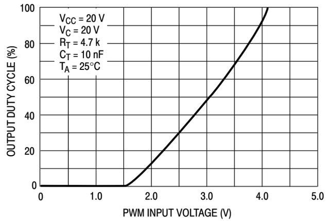
Figure 10. Output Duty Cycle versus PWM Input Voltage
