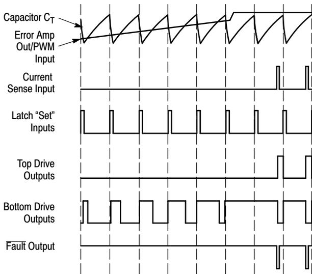
**Figure 21. Pulse Width Modulator Timing Diagram Reference**
