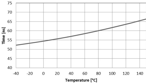
Figure 21.  $t_r$  for 10 nF Load vs. Temperature
