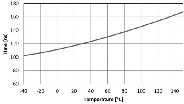
Figure 18.  $t_{OFF}$  vs. Temperature
