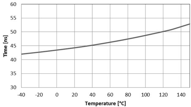
Figure 22.  $t_f$  for 10 nF Load vs. Temperature
