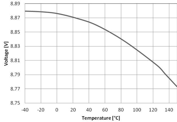
Figure 8. V<sub>Bon</sub> vs. Temperature
