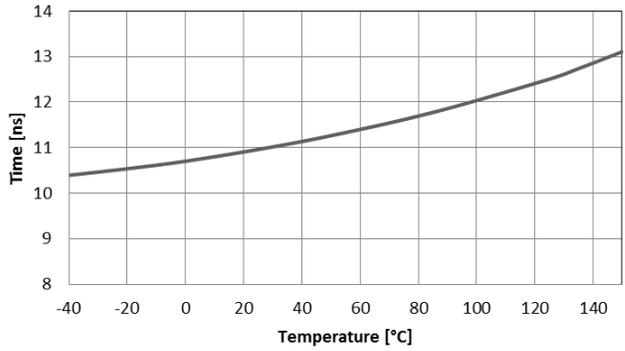
Figure 20.  $t_f$  vs. Temperature
