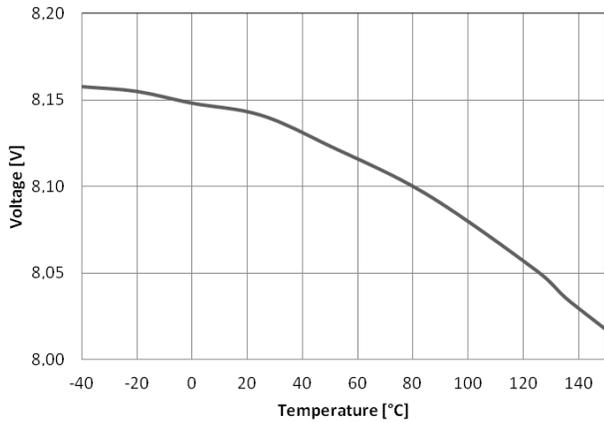
Figure 9. V<sub>Boff</sub> vs. Temperature
