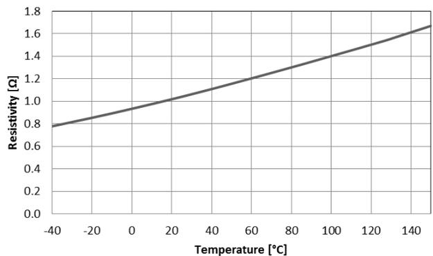
Figure 24.  $R_{OL}$  vs. Temperature
