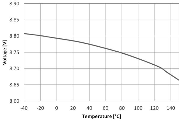
Figure 5. V<sub>CCOn</sub> vs. Temperature
