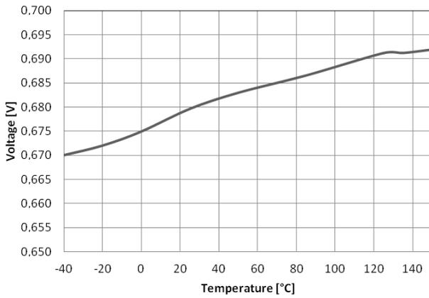
Figure 7. V<sub>CCUVLOHYS</sub> vs. Temperature
