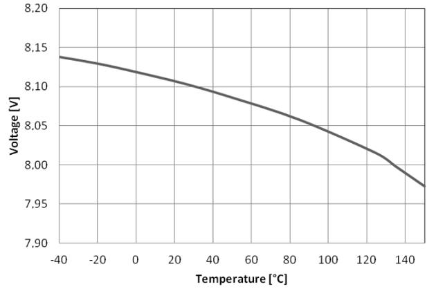
Figure 6. V<sub>CCOff</sub> vs. Temperature
