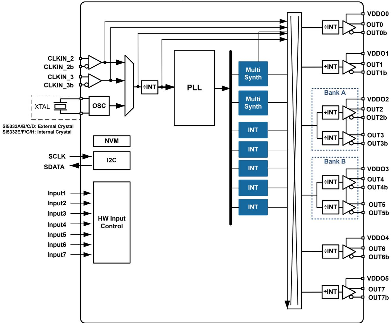
Figure 3.2. Block Diagram for 8-Output Si5332 in 40-QFN
