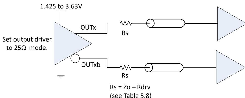
Figure 3.14. LVCMOS Output Termination Example, Option 2
