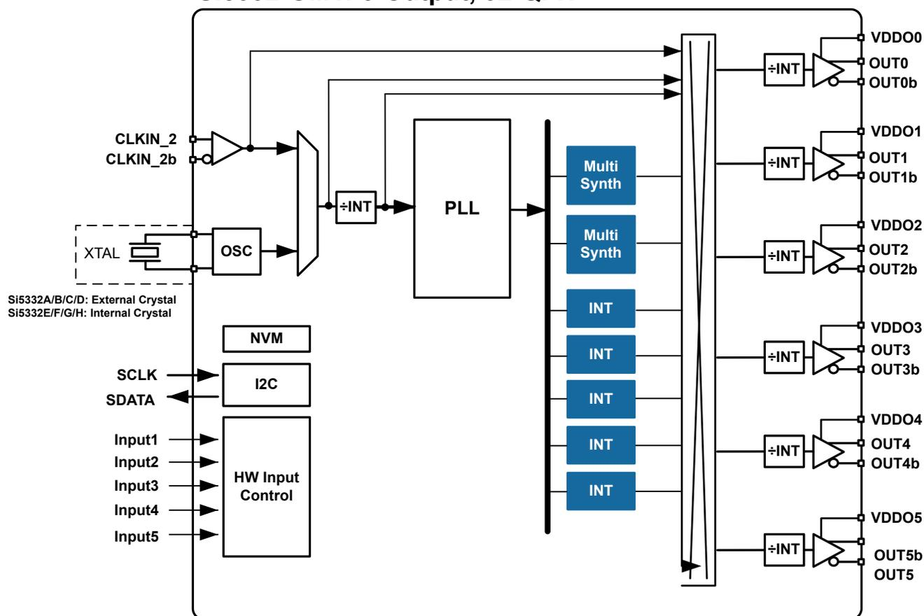
Figure 3.3. Block Diagram for 6-Output Si5332 in 32-QFN
