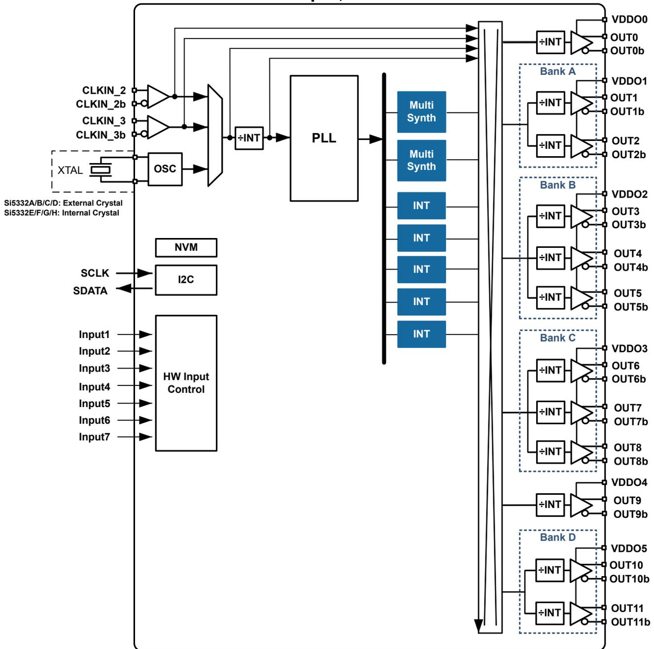
Figure 3.1. Block Diagram for 12-Output Si5332 in 48-QFN
