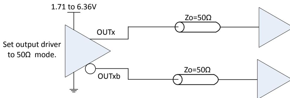
Figure 3.13. LVCMOS Output Termination Example, Option 1
