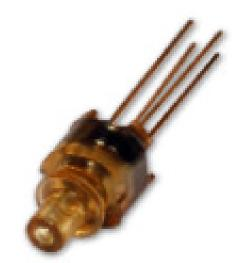
The HFD3180-108 use a high-performance GaAs PIN photo-detector packaged with a transimpedance amplifier designed to meet performance requirements for data rates up to 2.5Gbps data communication over multi-mode optical fiber at 850nm. Applications include Ethernet, Fiber Channel and ATM protocols. The optical assembly is designed to interface either 50mm or 62.5mm multi-mode fiber.
