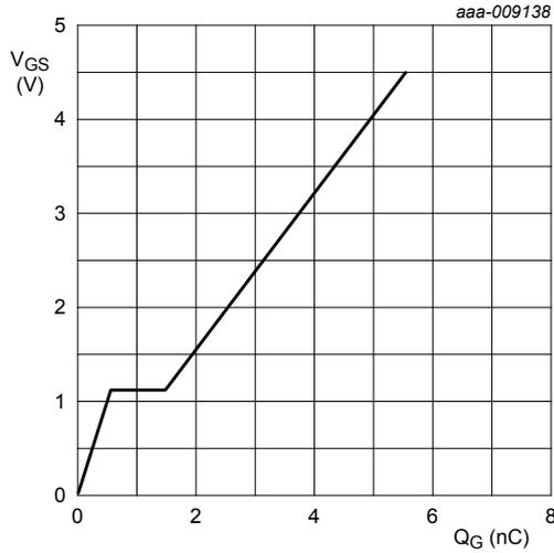
$I_D = 3.2$  A;  $V_{DS} = 10$  V;  $T_{amb} = 25$  °C
