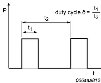
Fig. 18. Duty cycle definition
