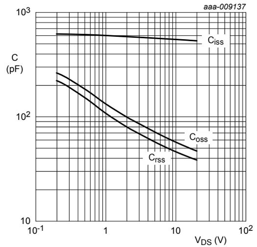
$$f = 1 \text{ MHz}; V_{GS} = 0 \text{ V}$$
