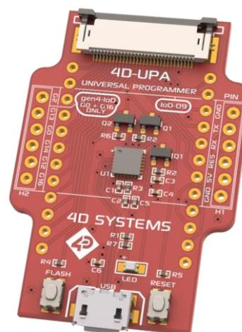
The 4D-UPA is a single module with microUSB interface, and DIP style pads for GPIO breakout of all the signals used on the Display interface, which is useful for development or final product use. Standard 2.54mm (0.1") male pin headers can be mounted so the module signals can be interfaced to easily.
