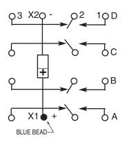
**NOTE:** Polarity must be observed with DC coil supply. Relay is polarized with a permanent magnet and will not operate or be damaged by reverse polarity.
