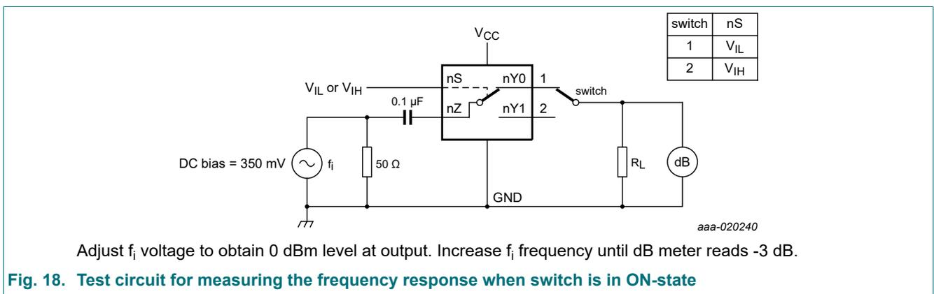
Adjust  $f_i$  voltage to obtain 0 dBm level at output. Increase  $f_i$  frequency until dB meter reads -3 dB.
