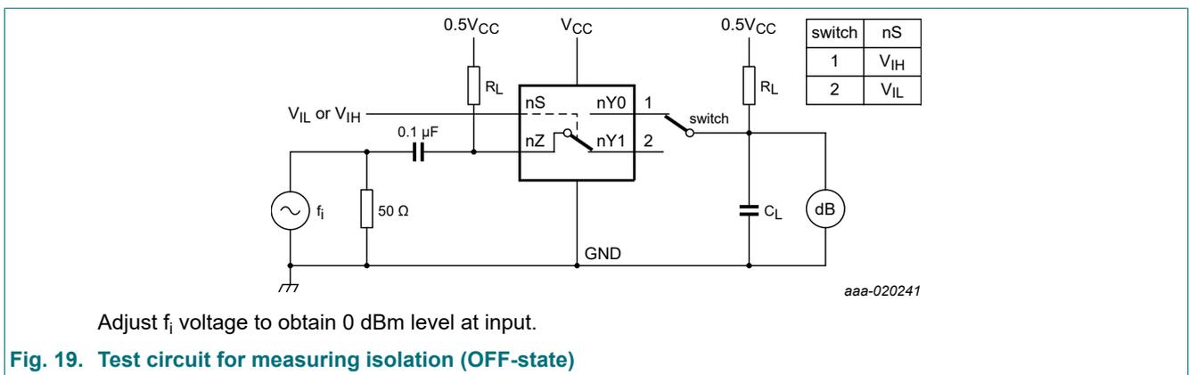
Adjust  $f_i$  voltage to obtain 0 dBm level at input.
