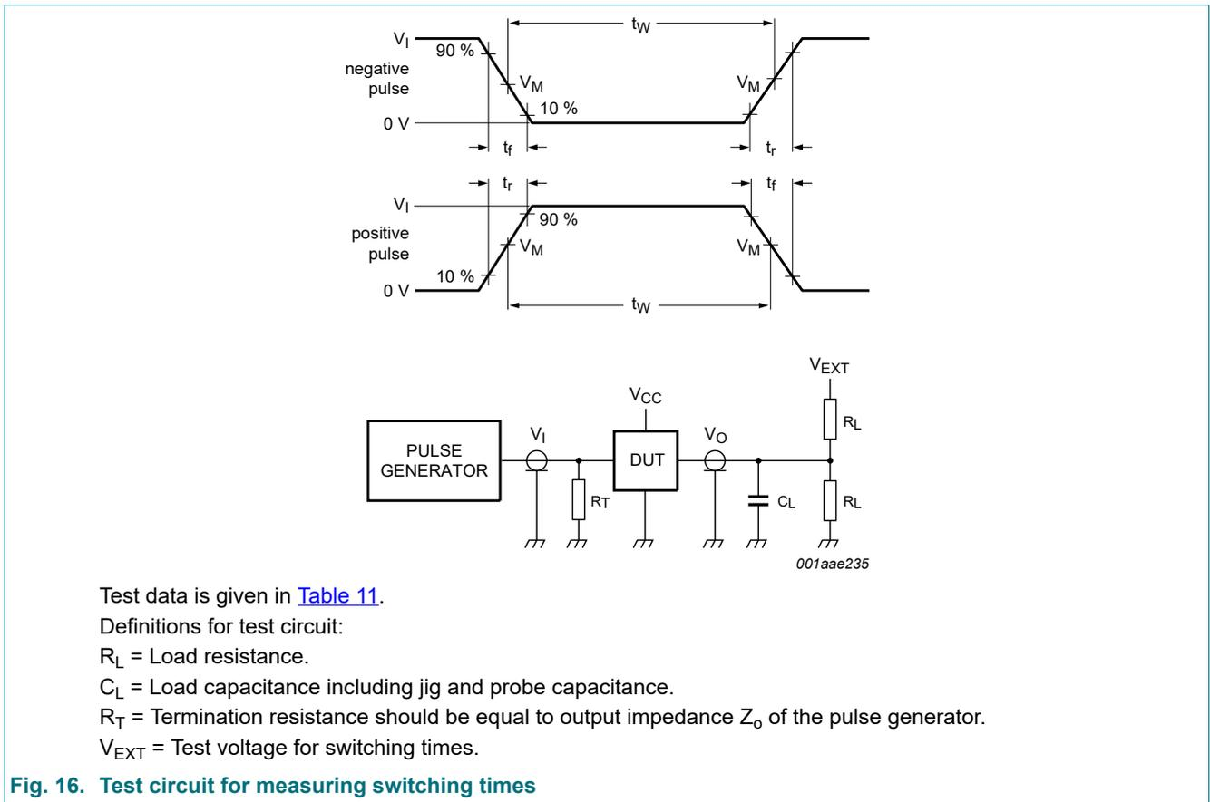
Fig. 16. Test circuit for measuring switching times
