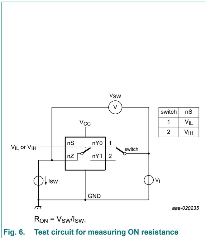
Fig. 6. Test circuit for measuring ON resistance
