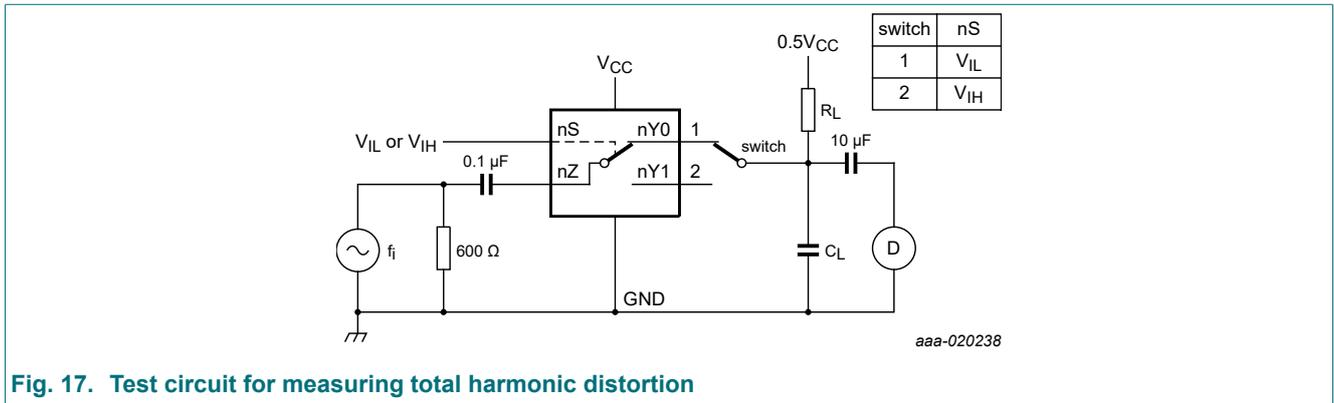
Fig. 17. Test circuit for measuring total harmonic distortion
