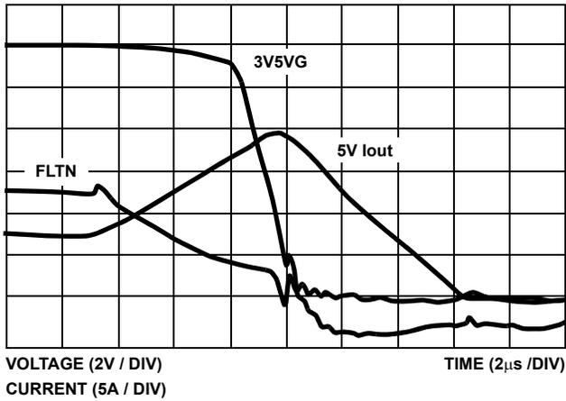
FIGURE 8. FLTN, 3V5VG RESPONSE TO OC, FLT<sub>N</sub> CAP = 0.01µF
