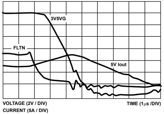
FIGURE 7. FLTN, 3V5VG RESPONSE TO OC, FLT<sub>N</sub> CAP = 0.001µF
