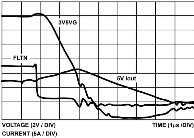
FIGURE 6. FLTN, 3V5VG RESPONSE TO OC, FLT<sub>N</sub> = 100pF
