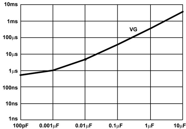
FIGURE 10. RESPONSE TIME vs FLT<sub>N</sub> CAP
