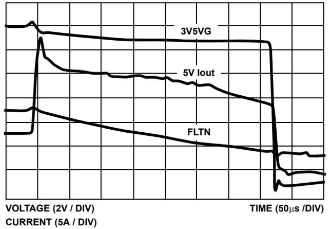
FIGURE 9. FLTN, 3V5VG RESPONSE TO OC, FLT<sub>N</sub> CAP = 1µF
