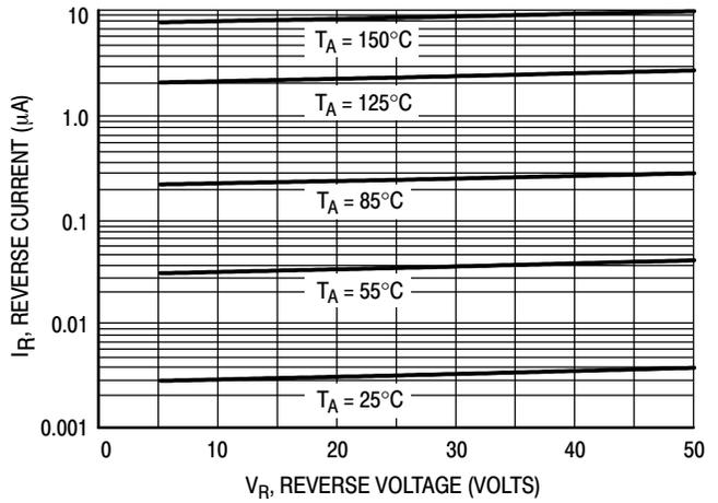
**Figure 3. Leakage Current**
