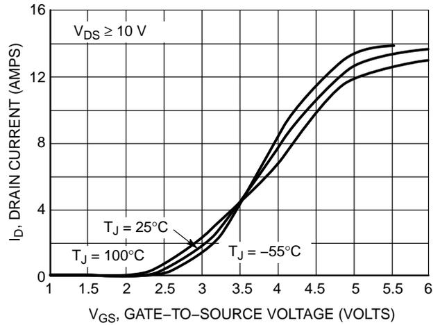
Figure 2. Transfer Characteristics
