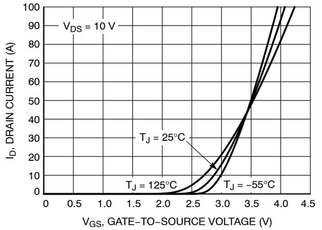
Figure 2. Transfer Characteristics
