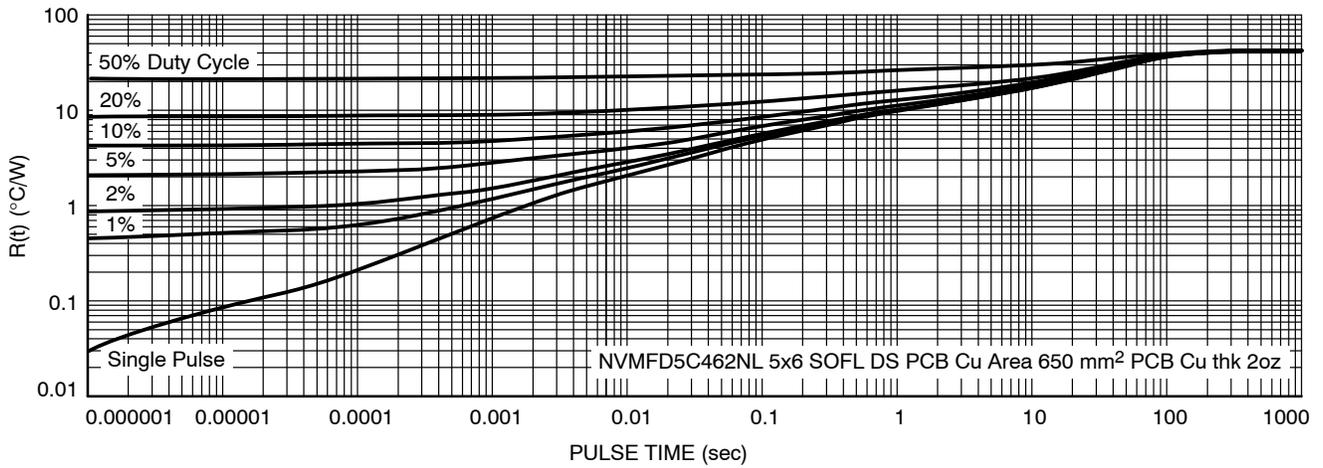
Figure 13. Thermal Characteristics
