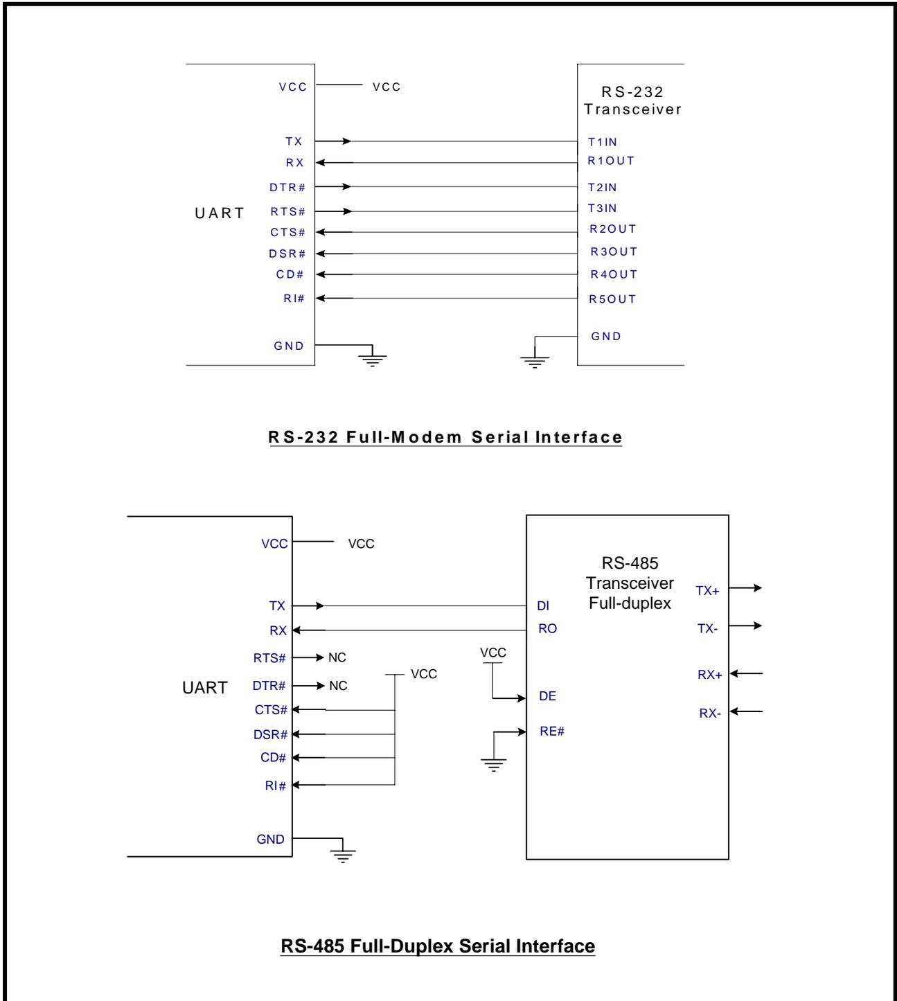
FIGURE 5. XR16M570 TYPICAL SERIAL INTERFACE CONNECTIONS
