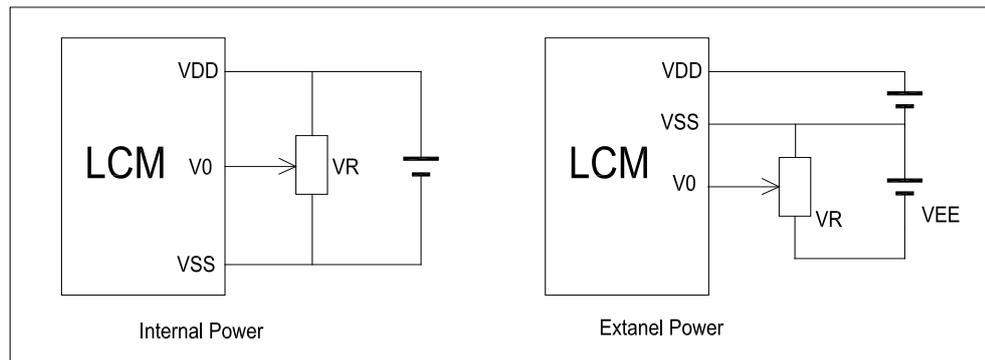
$V_{DD}-V_0$ : LCD Driving voltage
