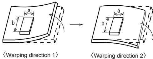
Products(warping direction 1, warping direction 2) shall be located carefully so that products are not subject to the mechanical stress due to warping the board. Because they may be subjected the mechanical stress in order of warping direction 1>warping direction 2.
