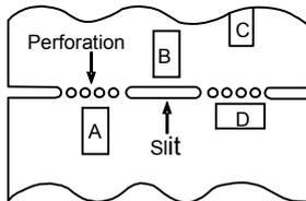
\*1  $A > D$  is valid when stress is added vertically to the perforation as with Hand Separation.
