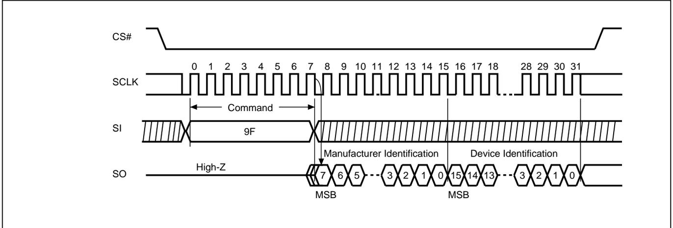
**Figure 26. Read Electronic Manufacturer & Device ID (REMS) Sequence (Command 90)**
