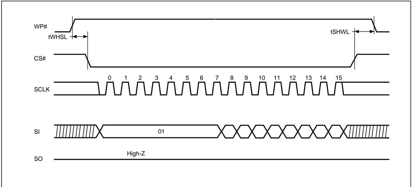
**Figure 11. Write Enable (WREN) Sequence (Command 06)**
