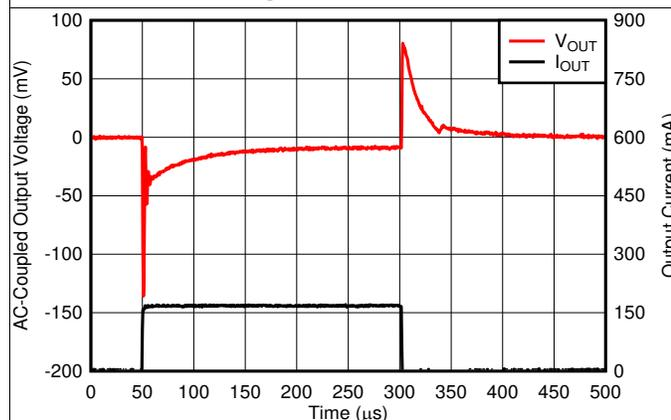
Figure 21. Load Transient
