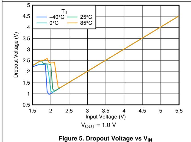
Figure 5. Dropout Voltage vs  $V_{IN}$
