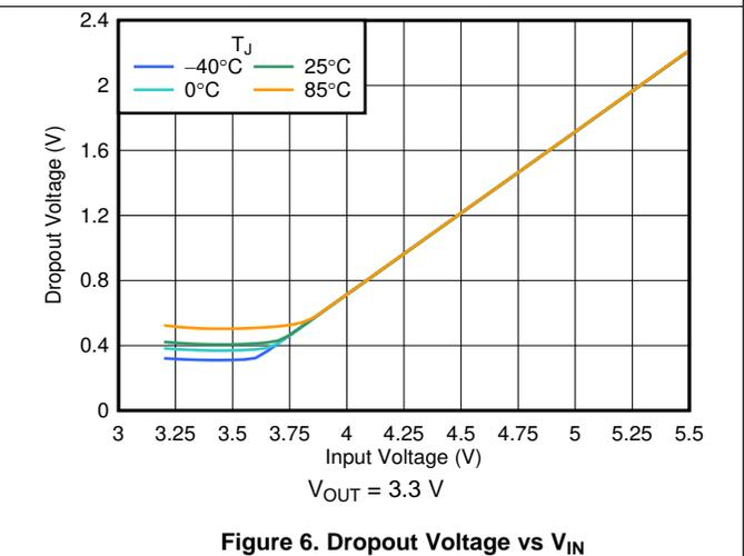
Figure 6. Dropout Voltage vs  $V_{IN}$
