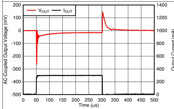
Figure 23. Load Transient
