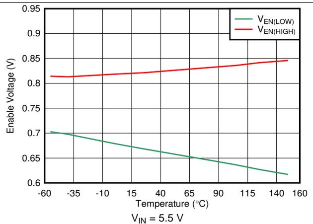
Figure 12. EN High and Low Threshold vs Temperature
