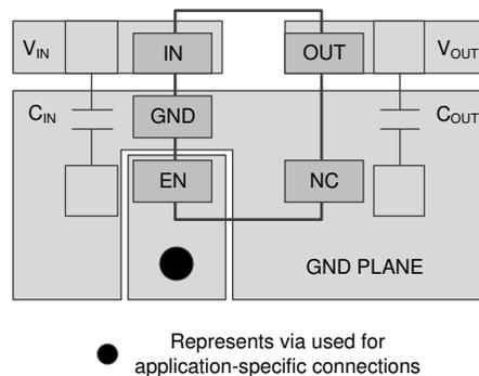
**Figure 38. Layout Example for the DBV Package**
