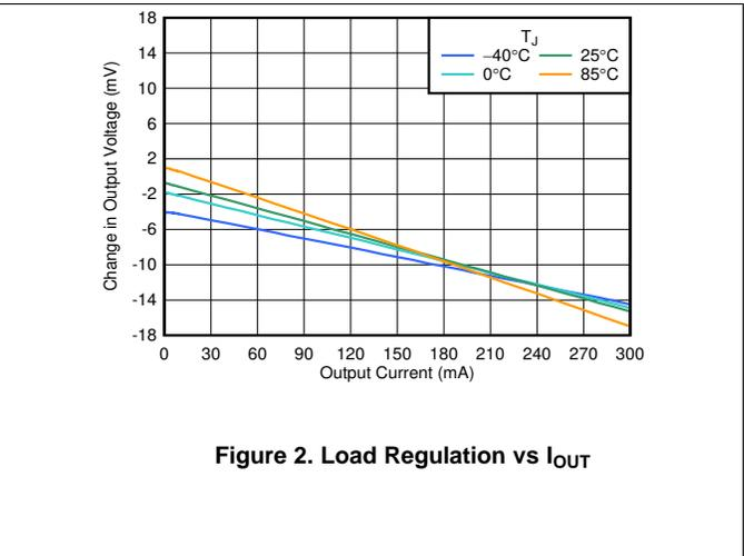
Figure 2. Load Regulation vs  $I_{OUT}$
