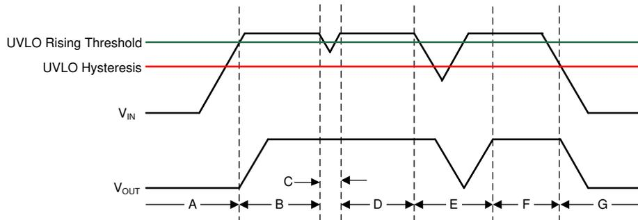
Figure 29. Typical UVLO Operation
