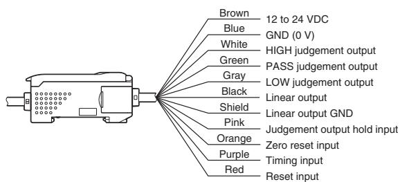
**Note 1.** Use a stabilized power supply separate from other devices and power systems for the Amplifier Unit, particularly when high resolution is required.
