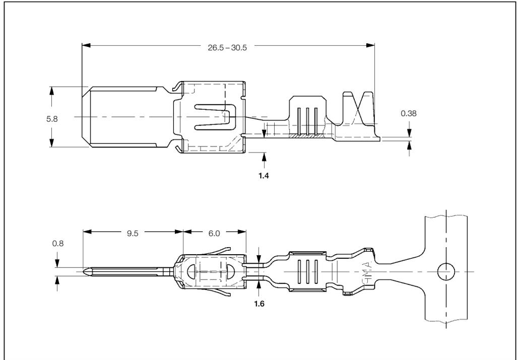
**Tab Contacts Single Wire Sealing System (SWS)**
