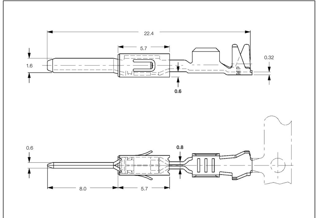
**Tab Contacts Single Wire Sealing System with Modified Spring (SWS)**
