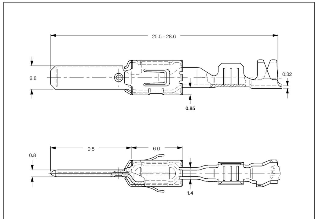
**Tab Contacts with Single Wire Sealing System (SWS)**
