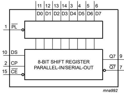
Fig. 3. Functional diagram
