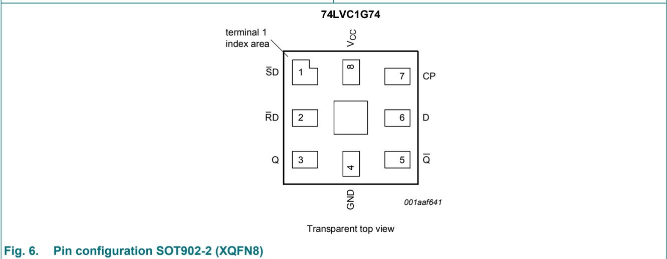
Fig. 6. Pin configuration SOT902-2 (XQFN8)
