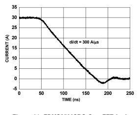
Figure 14. FDMS2506SDC SyncFET body diode reverse recovery characteristic
