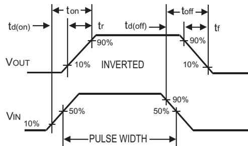
Figure 10. Switching Waveforms
