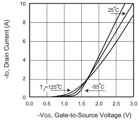
Figure 2. Transfer Characteristics
