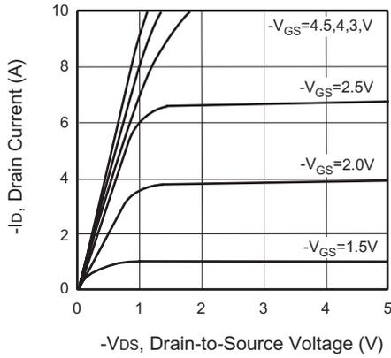
Figure 1. Output Characteristics
