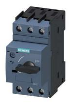
Circuit breaker size S00 for motor protection, CLASS 10 A-release 7...10 A N release 130 A screw terminal Standard switching capacity Multi-unit packaging Pack = 24 units
