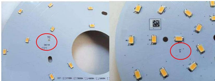
You can use the high-temperature thermal conductivity glue (Such as SatlonD-3/606...etc.) to fix the thermal couple to the  $T_c$  point then measure the temperature. Once you got the  $T_c$  temperature measurement data, you can calculate the junction temperature based on the measurement data of the  $T_c$ .
