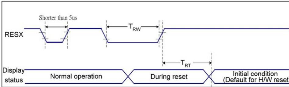
**Figure 7 Reset Timing**
