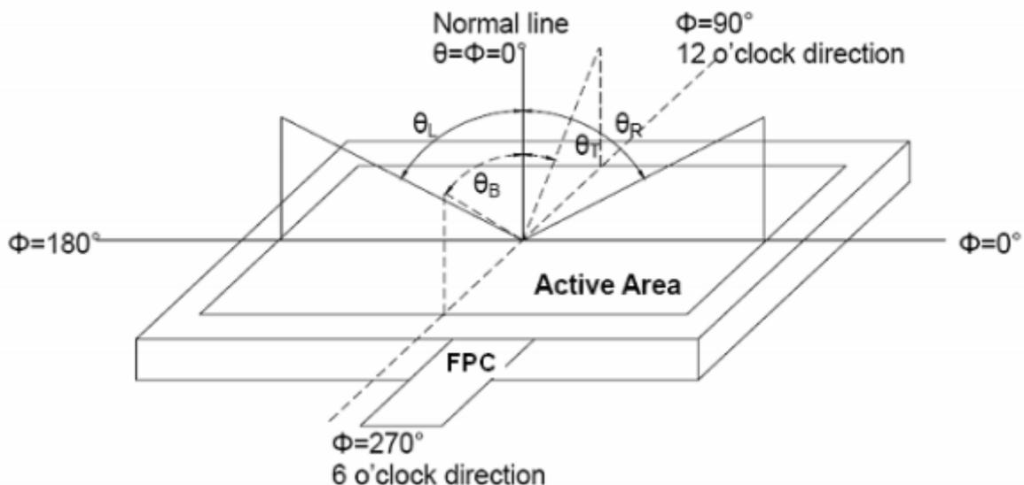
FIG. 3 The definition of Viewing Angle
