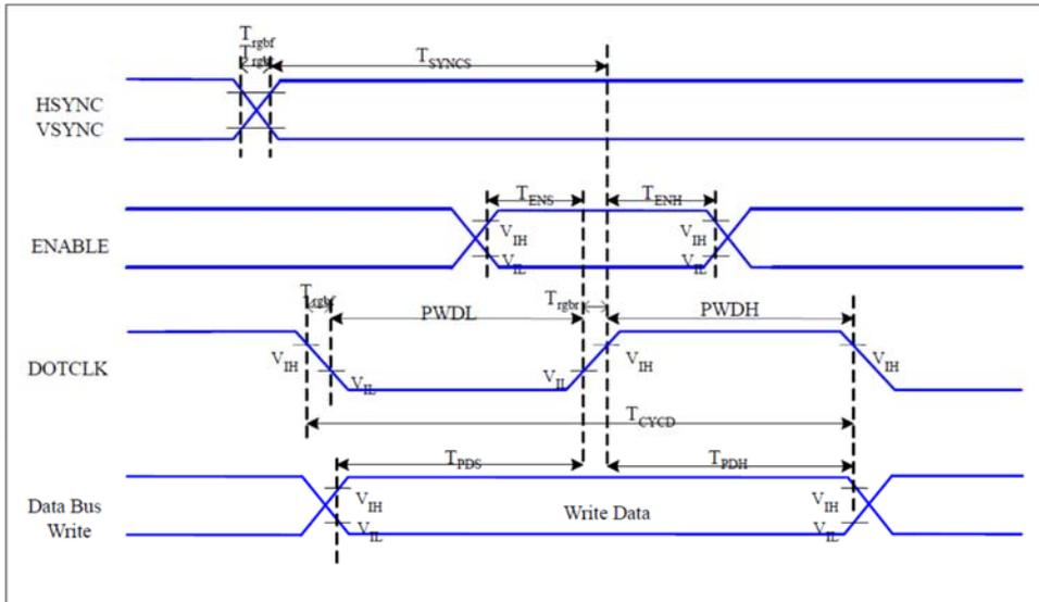
**Figure 6 RGB Interface Timing Characteristics**
