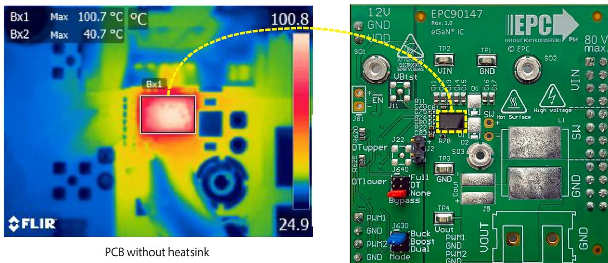
Figure 16: Measured thermal image showing the case temperature when operating under the following conditions:  $f_s = 500 \text{ kHz}$ ,  $I_{OUT} = 23 \text{ A}$  output, 25°C ambient and high airflow
