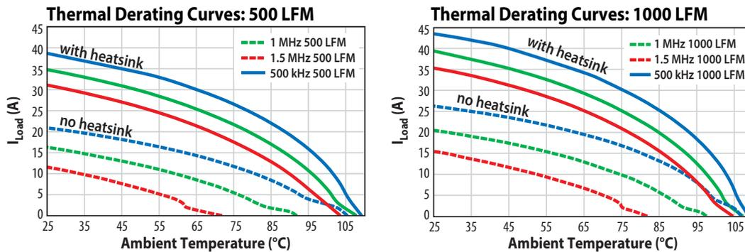
Figure 19: Typical thermal derating curve for two air flow rates, with and without a heatsink attached, measured with the board operating at various switching frequencies and using a 2.2 μH inductor
