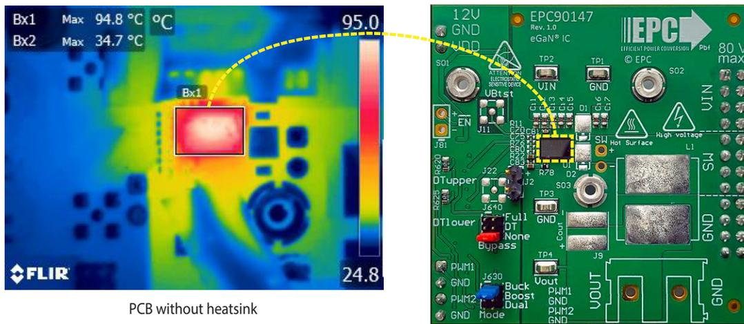
Figure 18: Measured thermal image showing the case temperature when operating under the following conditions:
