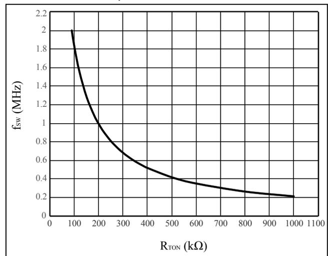
Figure 30 Operating Frequency vs. R<sub>TON</sub> Resistance
