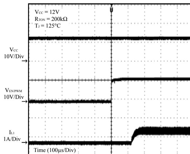
**Figure 20** EN/PWM Enable Time
