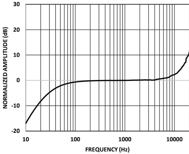
Figure 4. Typical Audio Frequency Response, High Quality Mode
