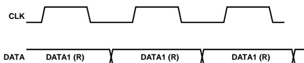
**Figure 10. Mono PDM Format**
