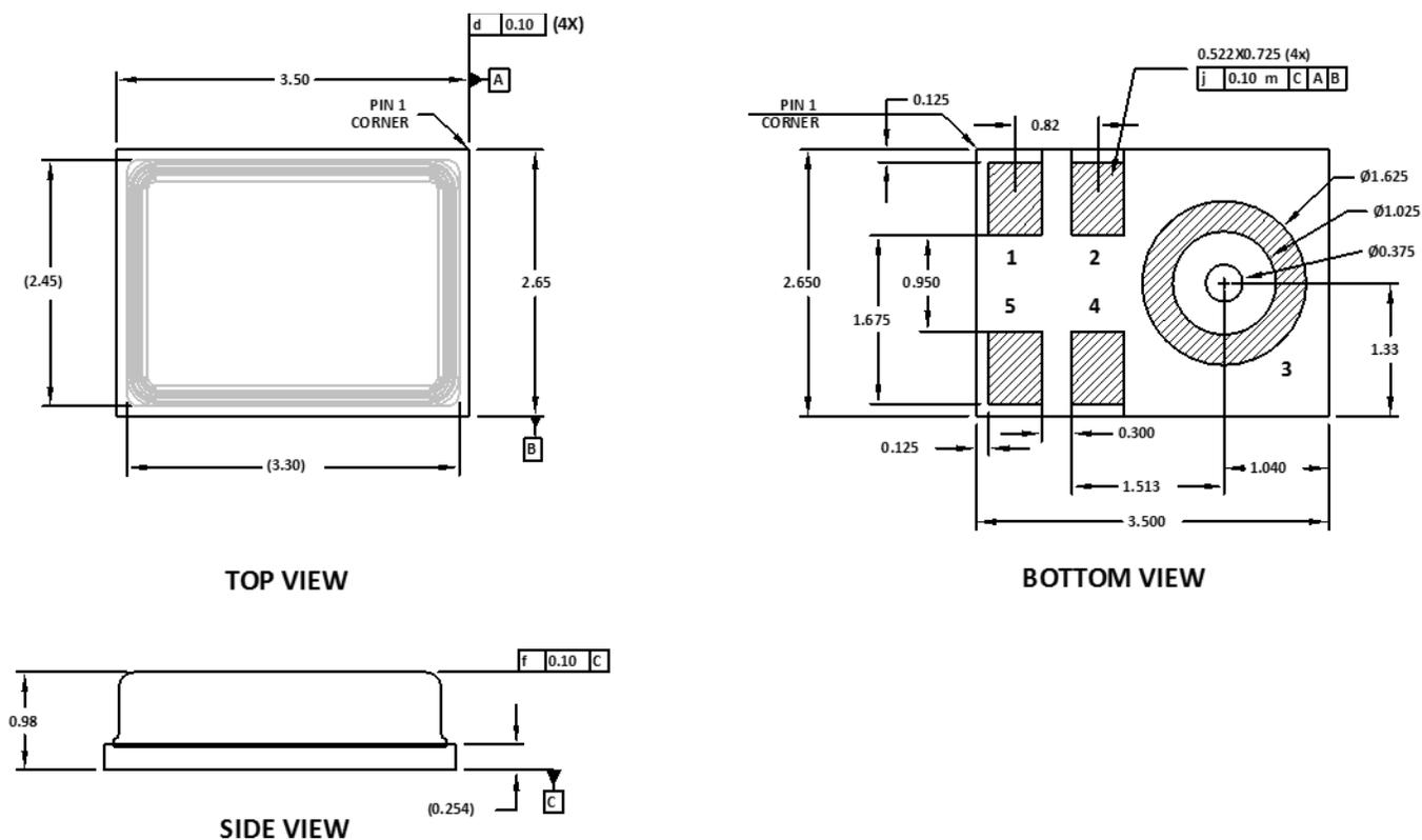
**Figure 17. 5-Terminal Chip Array Small Outline No Lead Cavity [LGA\_CAV]
