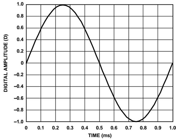
**Figure 11. 1 kHz, 0 dB FS Sine Wave**
