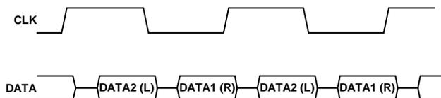
**Figure 9. Stereo PDM Format**
