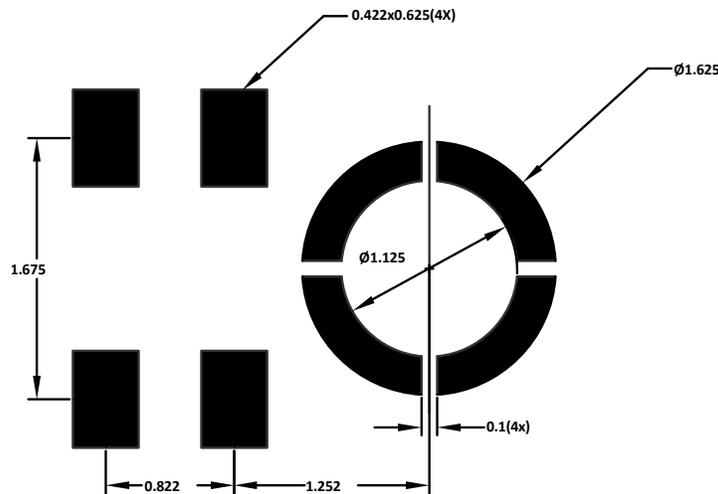
**Figure 16. Suggested Solder Paste Stencil Pattern Layout**
