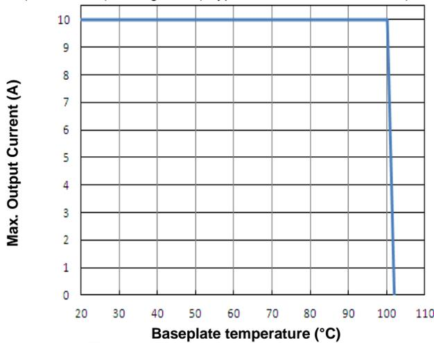
**Figure 11. Current Derating Curve for Baseplate**
