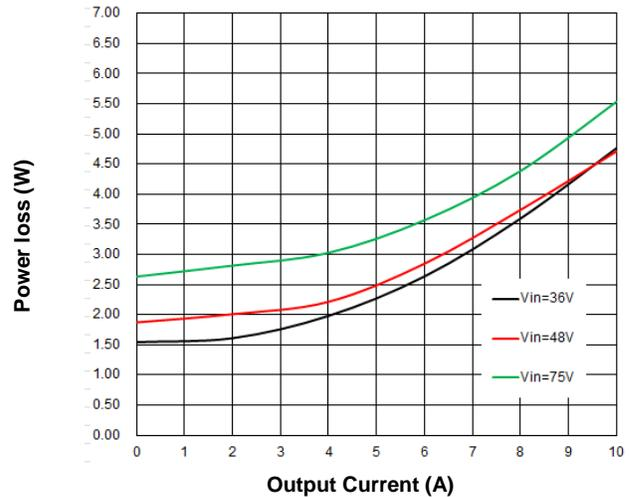
Figure 2. Power loss vs. Output Current (25°C)
