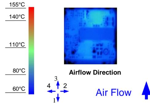
**Figure 10. Thermal Image for Airflow Direction 3**
