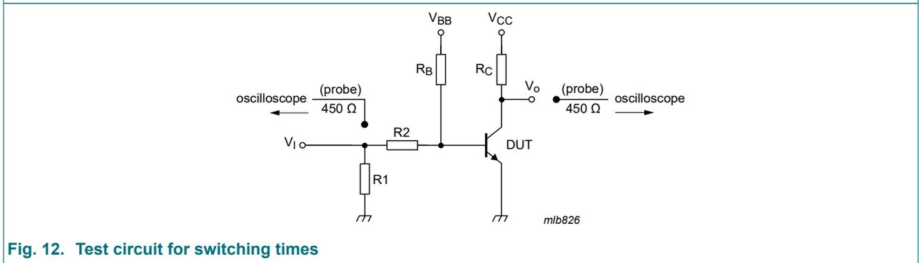
Fig. 12. Test circuit for switching times
