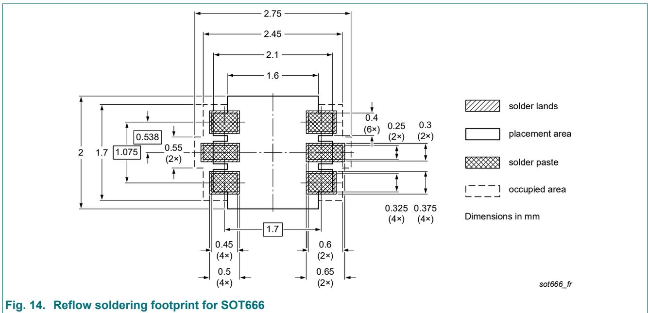
Fig. 14. Reflow soldering footprint for SOT666
