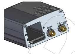
After removing the end-plate, the IoT slot (and SIM slot) can be accessed
