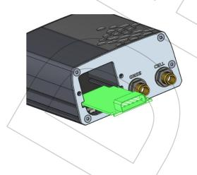
Carefully line up the IoT card with the slots in the aluminium extrusion.
