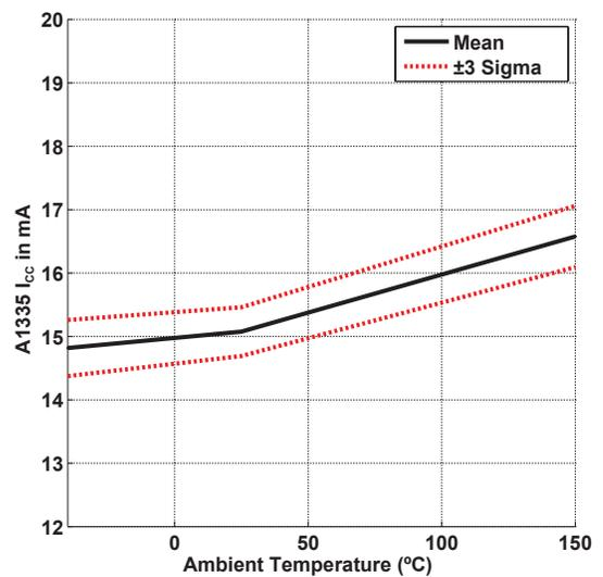
Figure 26: I<sub>CC</sub> over Temperature
