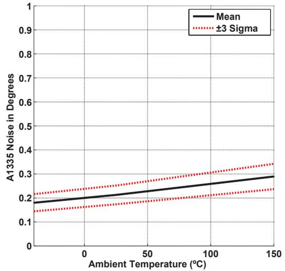
Figure 24: Noise Performance over Temperature
