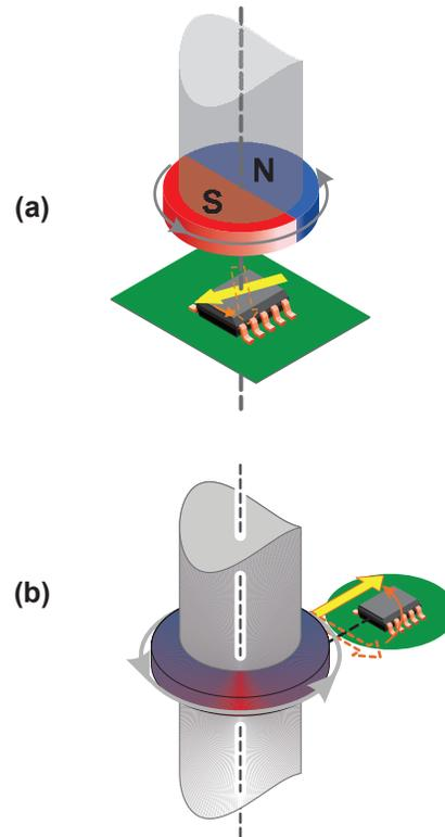
**Figure 12: Typical On-Axis (a) and Off-Axis (b) Orientation**
