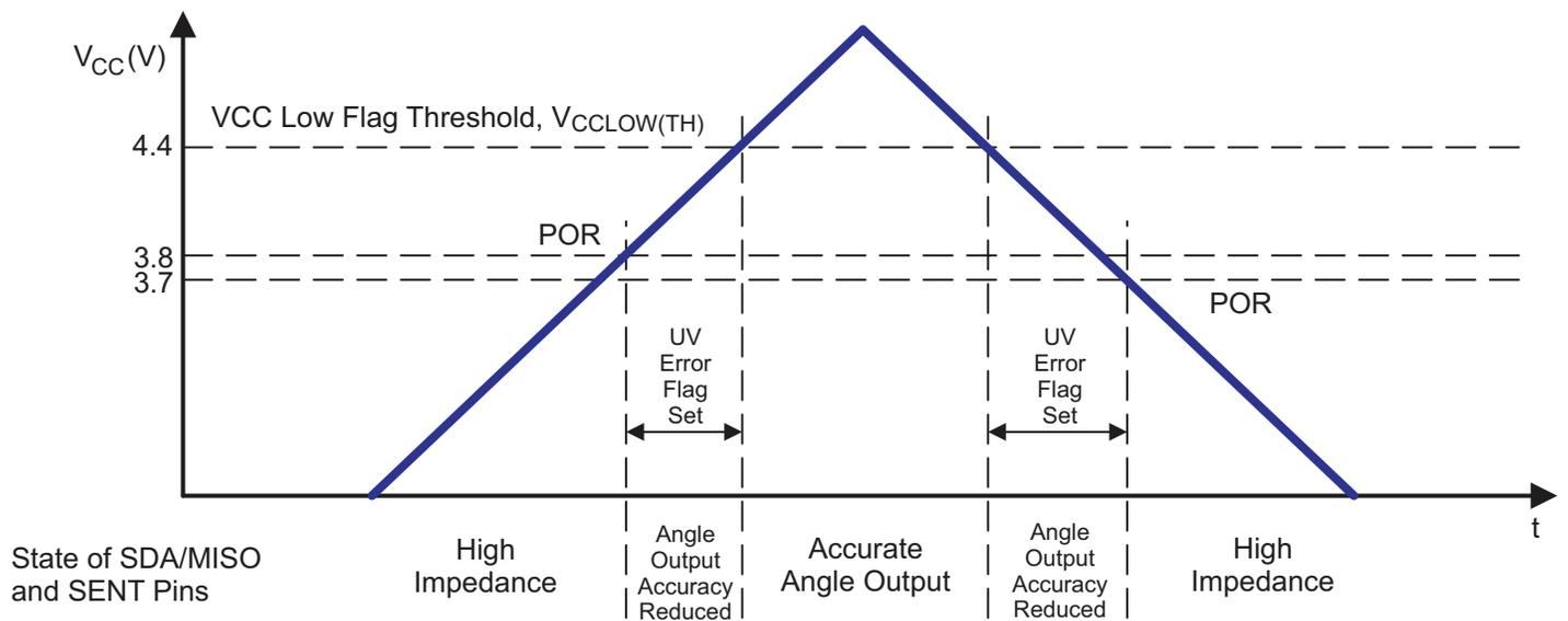
Figure 2: Relationship of V<sub>CC</sub> and Output
