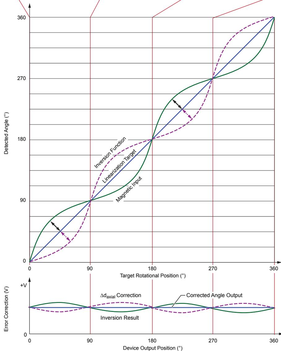
Figure 18b: Any eccentricity is evaluated as an error. Systematic eccentricity can be factored out by appropriate linearization coefficients. For off-axis applications, the harmonic linearization method is recommended.
