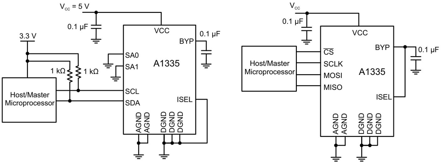
**(A) Typical A1335 configuration using I<sup>2</sup>C interface; A1335 set up for serial address 0xC**
