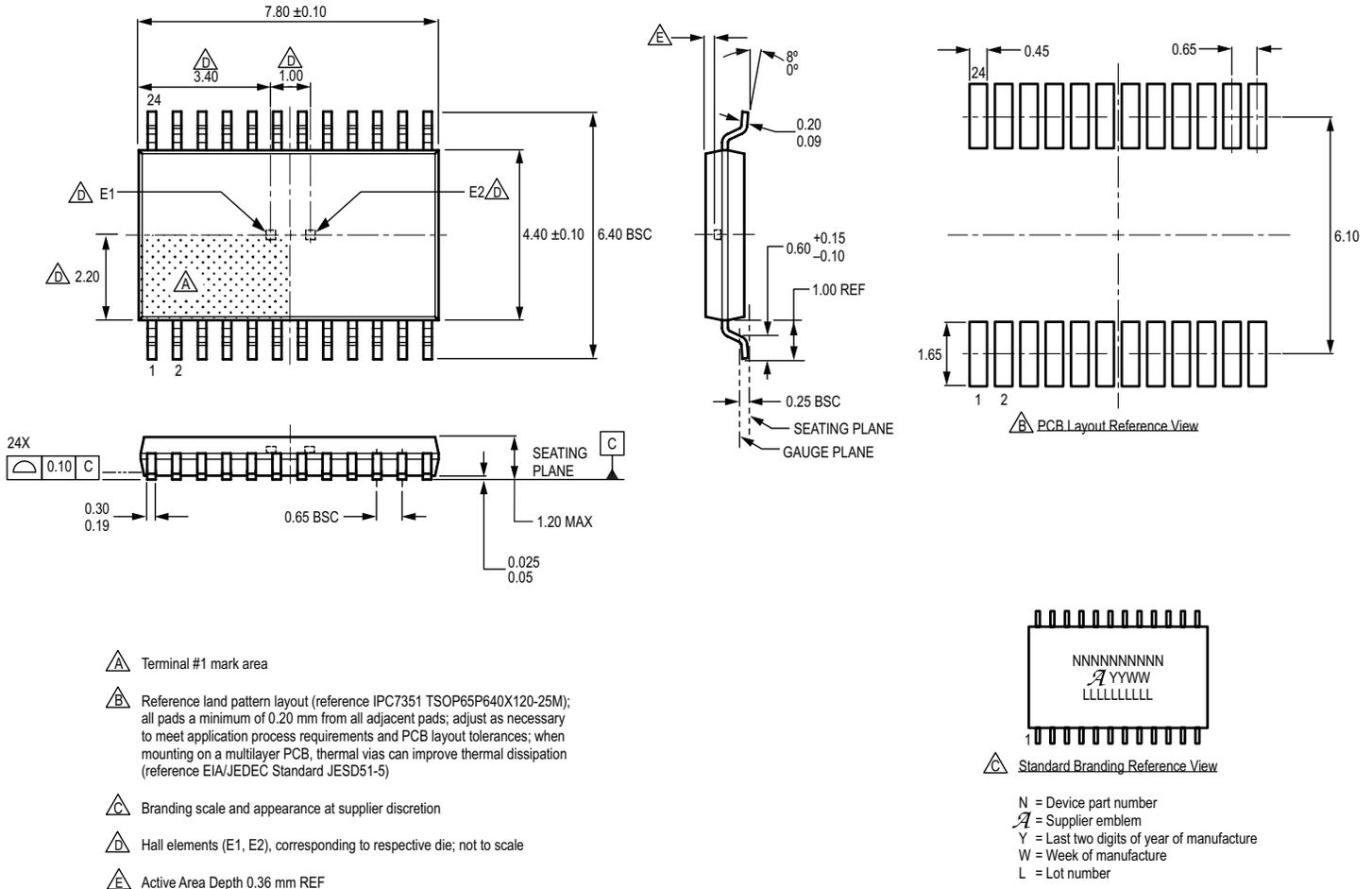
Figure 28: Package LE, 24-Pin TSSOP (Dual Die Version)
