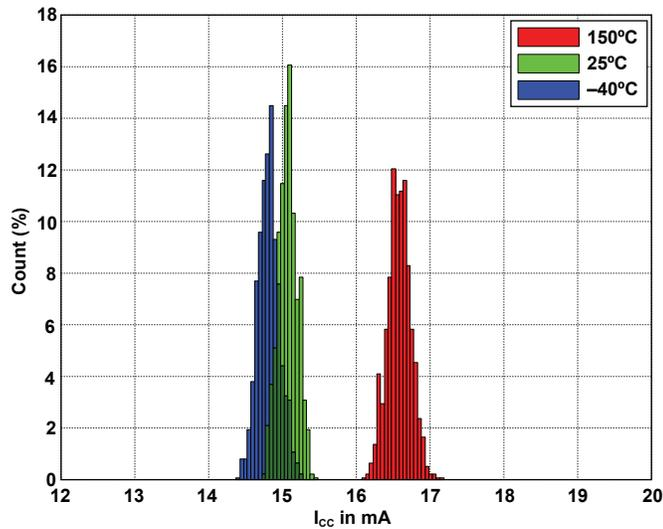
Figure 25: I<sub>CC</sub> Distribution over Temperature
