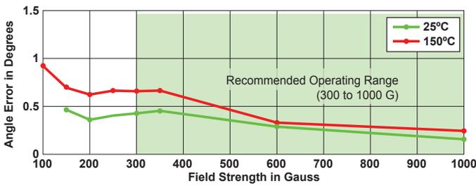
**Figure 9: Typical Maximum Angle Error Over Field Strength**
