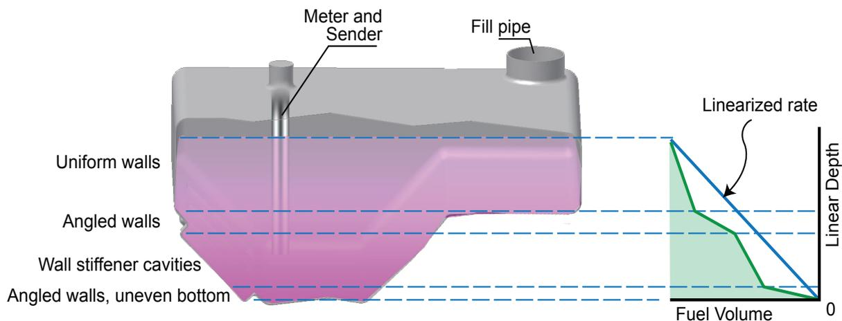
**Figure 17: An integrated vehicle fuel tank has varying volumes according to depth due to structural elements. As shown in the chart, this results in a variable rate of fuel level change, depending on volume at the given depth, and a linearized transfer function can be used against the integral volume.**
