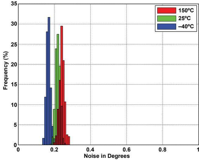
Figure 23: Noise Distribution over Temperature
