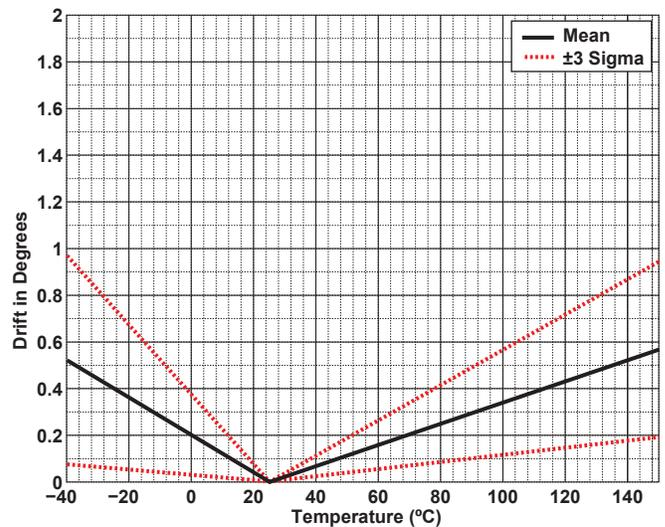
Figure 22: Maximum Absolute Drift from 25°C Reading (300 G)
