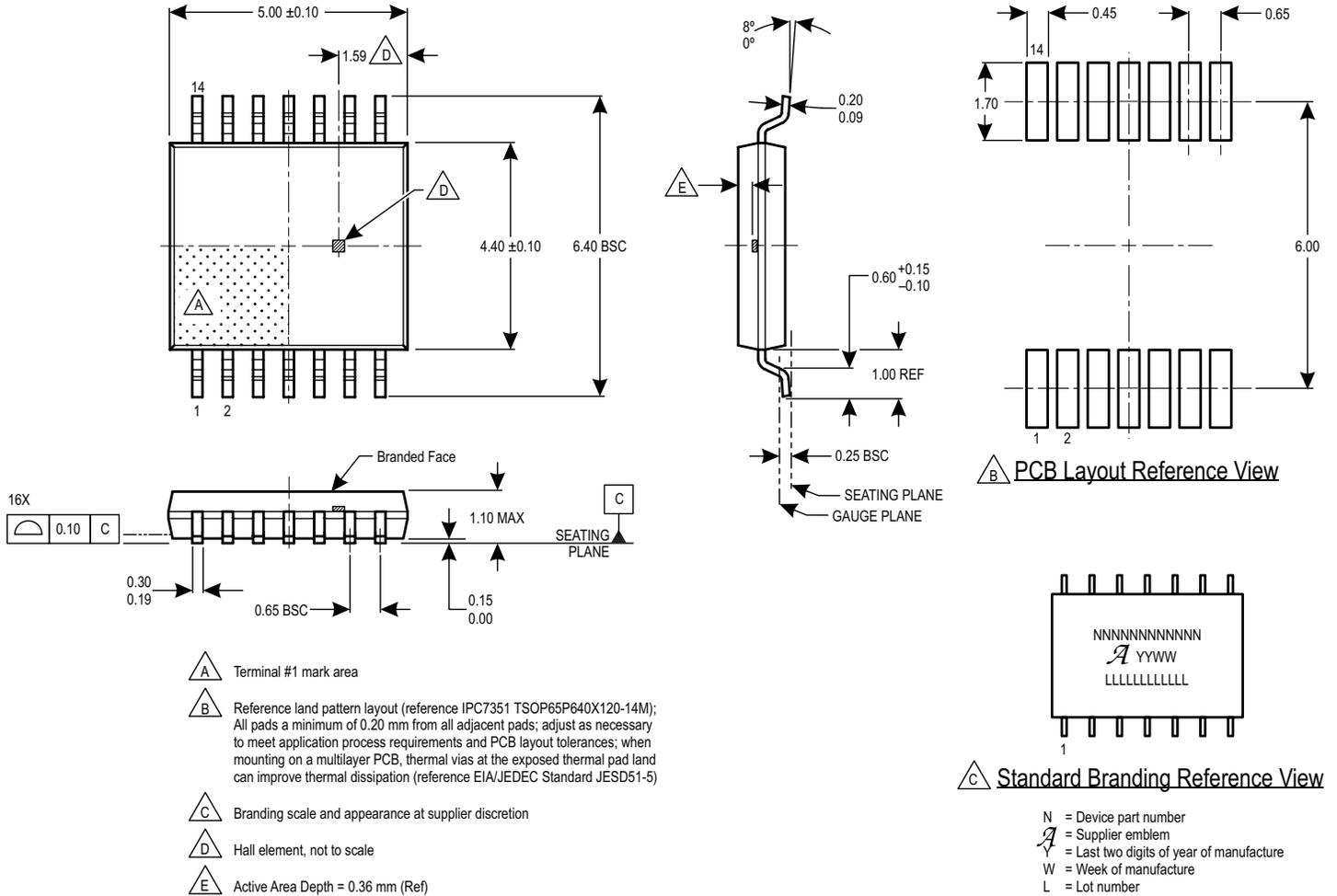
Figure 27: Package LE, 14-Pin TSSOP (Single Die Version)
