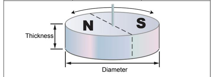
\*A sintered Neodymium magnet with 10 mm (or greater) diameter and 4 mm thickness is the recommended magnet for redundant applications.
