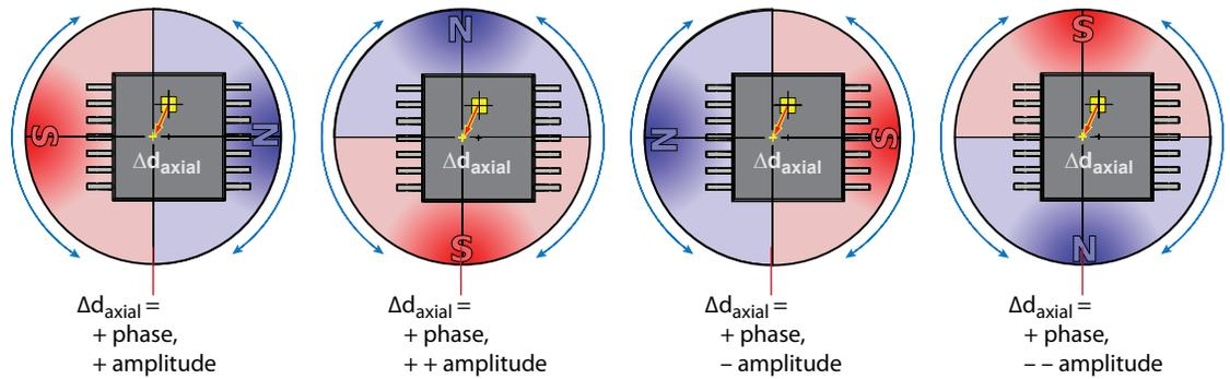
Figure 18a: With the axis of rotation aligned with the Hall element, linearization coefficients are a simple inversion of the input.
