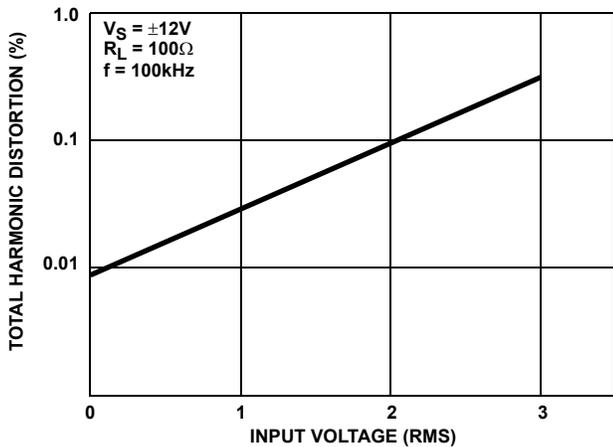
FIGURE 22. TOTAL HARMONIC DISTORTION vs INPUT VOLTAGE
