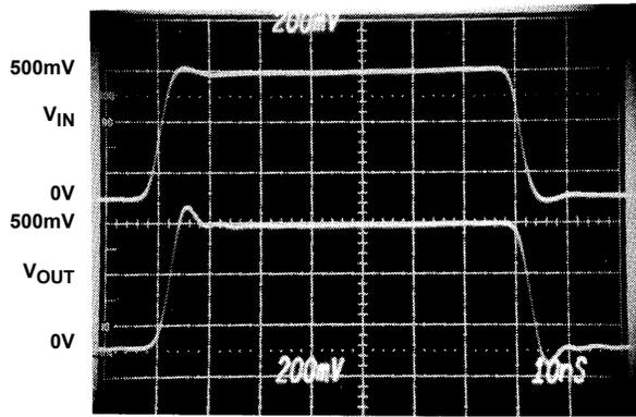
$T_A = 25^\circ\text{C}$ ,  $R_S = 50\Omega$ ,  $R_L = 100\Omega$
