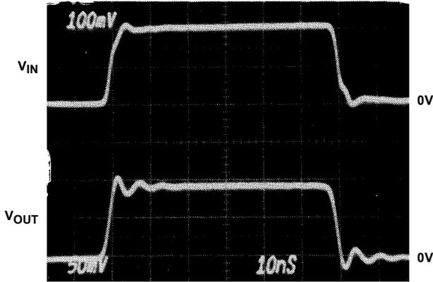
$T_A = 25^\circ\text{C}$ ,  $R_S = 50\Omega$ ,  $R_M = R_L = 50\Omega$
