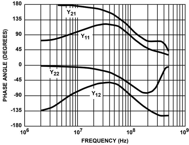
FIGURE 18. Y - PARAMETERS PHASE vs FREQUENCY
