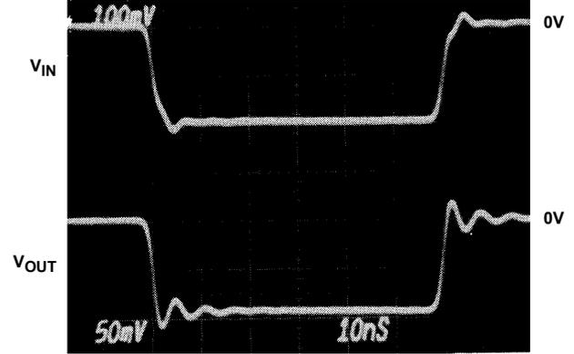
$T_A = 25^\circ\text{C}$ ,  $R_S = 50\Omega$ ,  $R_M = R_L = 50\Omega$
