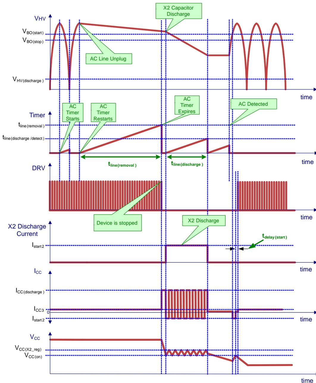
Figure 21. Line Removal Timing with AC Reapplied
