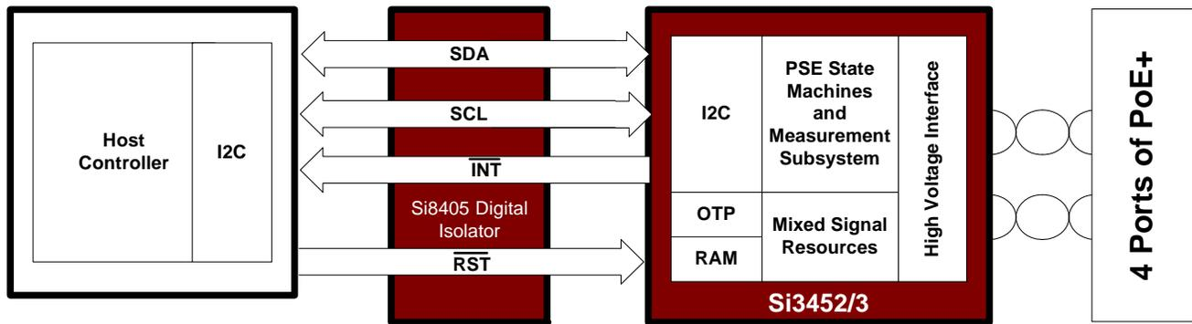
Figure 2. 4-Port System with Direct Host Connection
