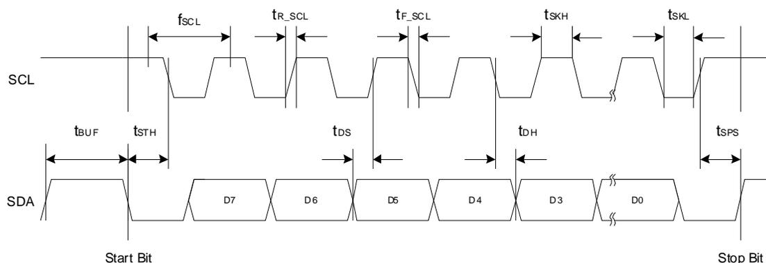
Figure 1. I<sup>2</sup>C Timing DiagramTable 12. Interrupt ( $\overline{\text{INT}}$ ) Specifications
