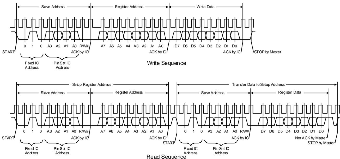
**Figure 6. Typical I<sup>2</sup>C Bus Transactions**
