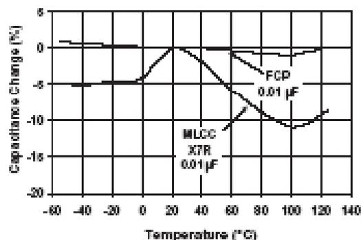
The capacitance of SMT film chips is much more stable with applied voltage and with changes in temperature than multilayer ceramic capacitors. Add in the low ESR characteristics of film chips and the final result is improved performance in filter circuit applications.
