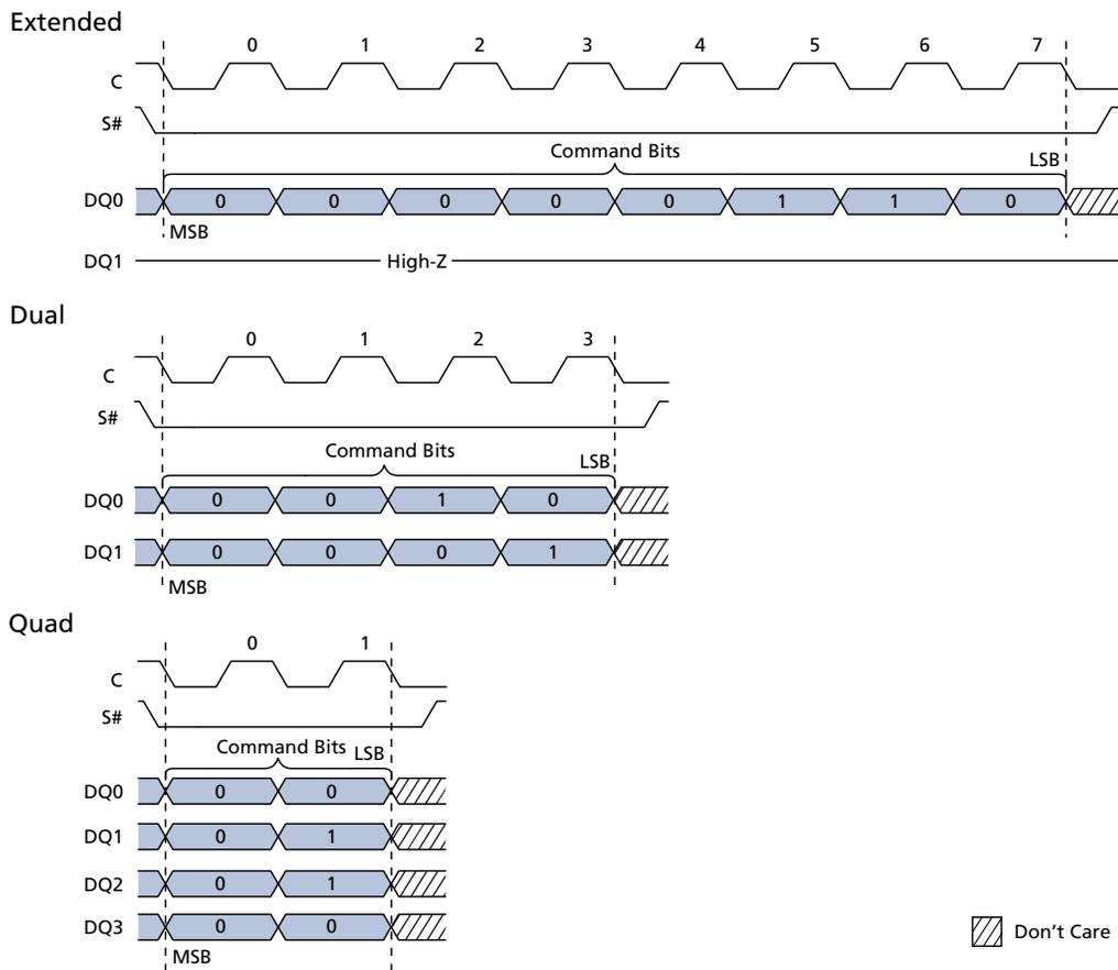
Note: 1. WRITE ENABLE command sequence and code, shown here, is 06h (0000 0110 binary); WRITE DISABLE is identical, but its command code is 04h (0000 0100 binary).
