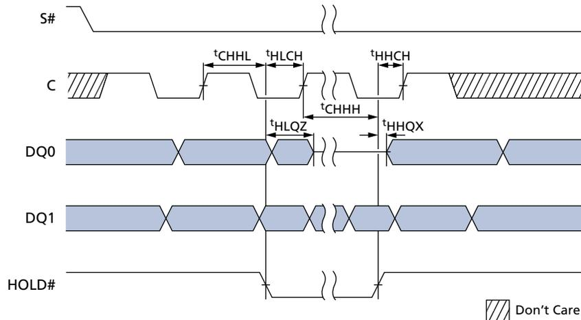
Figure 56: Output Timing for STR
