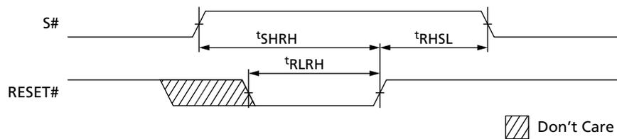
**Figure 51: Reset Enable and Reset Memory Timing**
