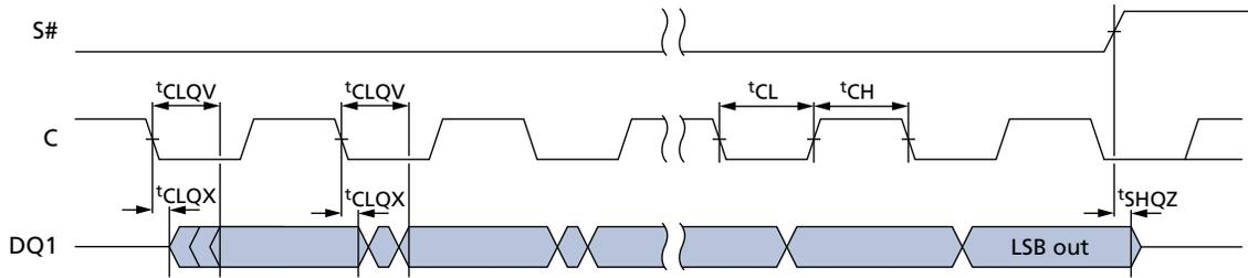
Figure 57: Output Timing for DTR
