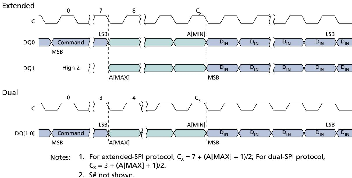
**Figure 38: QUAD INPUT FAST PROGRAM Command**
