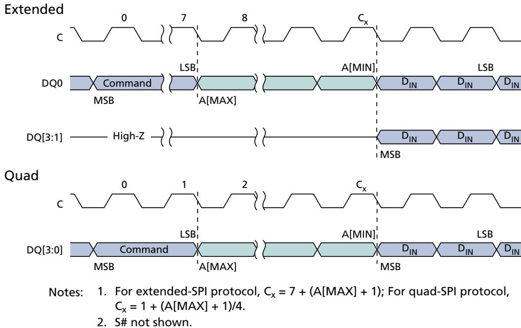
**Figure 39: EXTENDED QUAD INPUT FAST PROGRAM Command**
