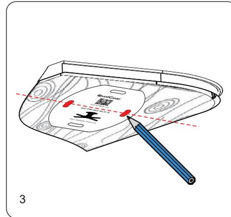
Using the marking template provided, mark two holes for drilling on the centerline of the stud.
