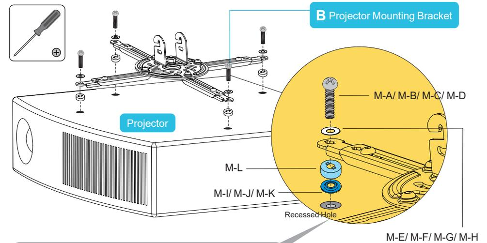
**NOTE** Choose the appropriate spacer (M-I/ M-J/ M-K) when mounting to recessed holes.
