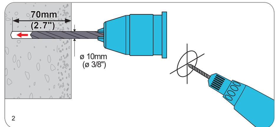
Using a power drill and a 3/8" masonry drill bit, drill mounting holes of 3/8" (10 mm) diameter and 2.7" (70 mm) depth at the marked locations in the previous step.
