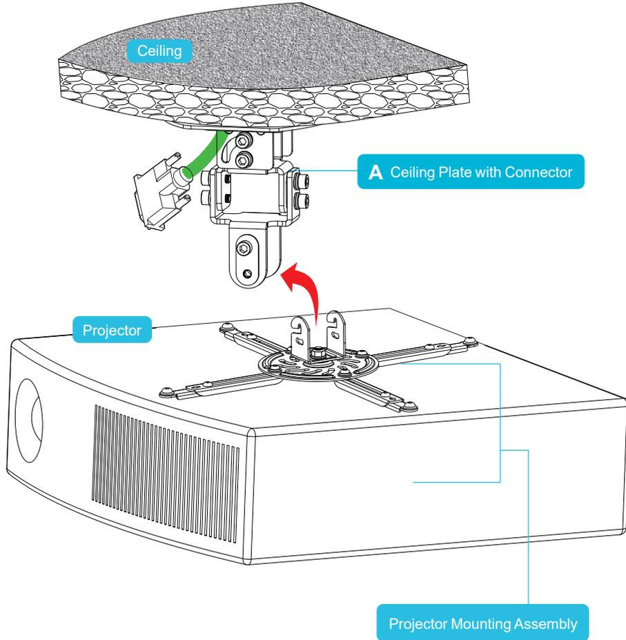
Align the Projector Mount Assembly to the Ceiling Plate with Connector, then using the Alley Key (M-P), attach them together with the provided Screws (M-M), Washers (M-N), and Plastic Washers (M-O).
