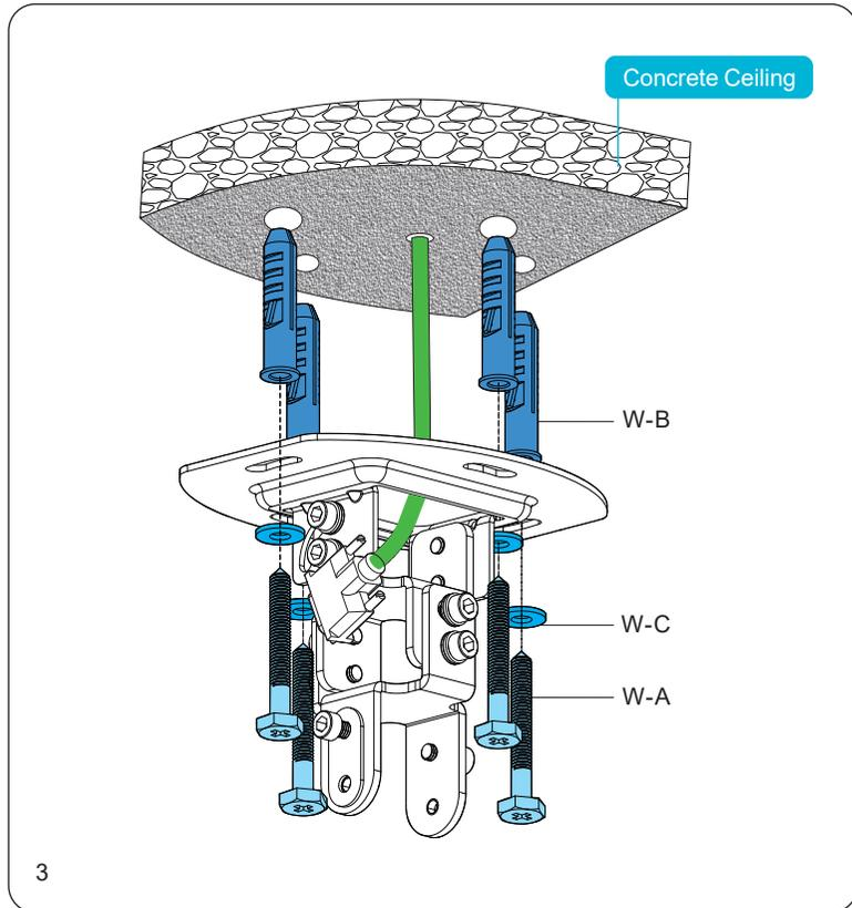
Place plastic anchors (W-B) in each hole. Tap each anchor flush with the ceiling using a hammer. Using a socket wrench, mount the ceiling plate and fasten with the provided lag bolts (W-A) and D6 washers (W-C).
