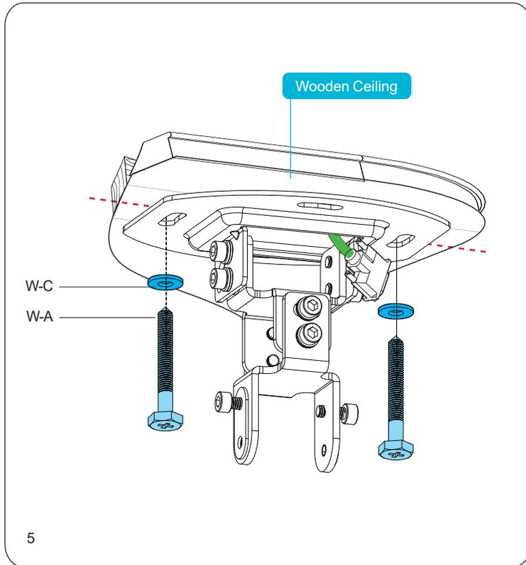
Using a socket wrench, mount the ceiling plate and fasten with the provided lag bolts (W-A) and D6 washers (W-C).
