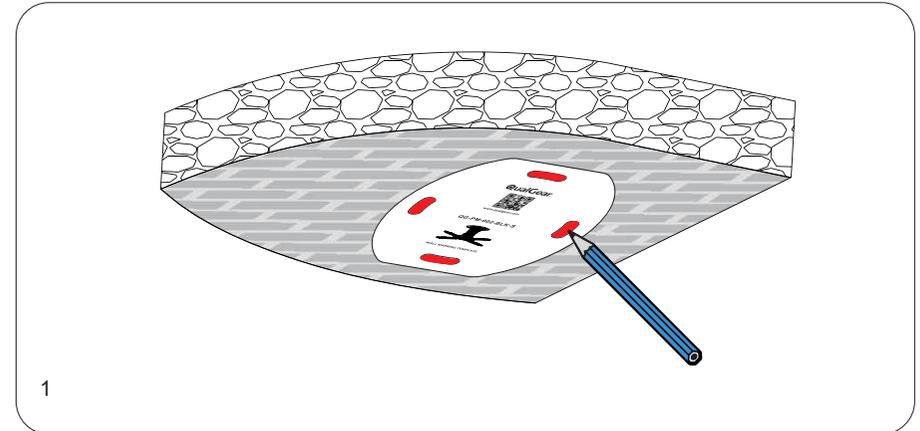
Hold the marking template provided against the ceiling where you want to install the projector, mark four holes for drilling.
