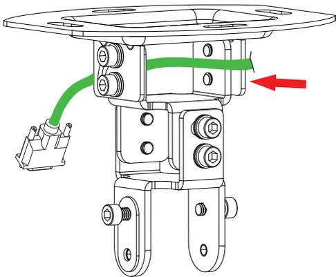
Feed the projector cable(s) through the side of the Ceiling Plate.
