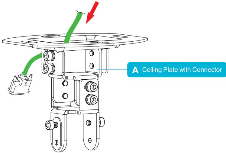
Feed the projector cable(s) through the top of the Ceiling Plate.
