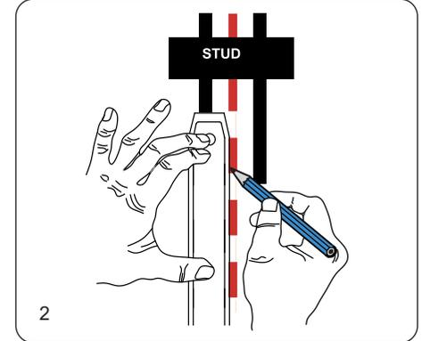
Using a straight edge, mark the centerline of the stud.
