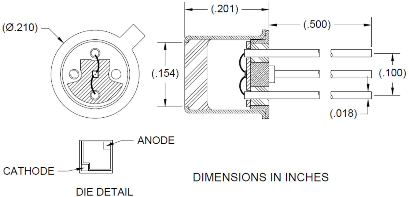
>Soldering Conditions: 260°C 1/16 inch away from case for 3 seconds max.
