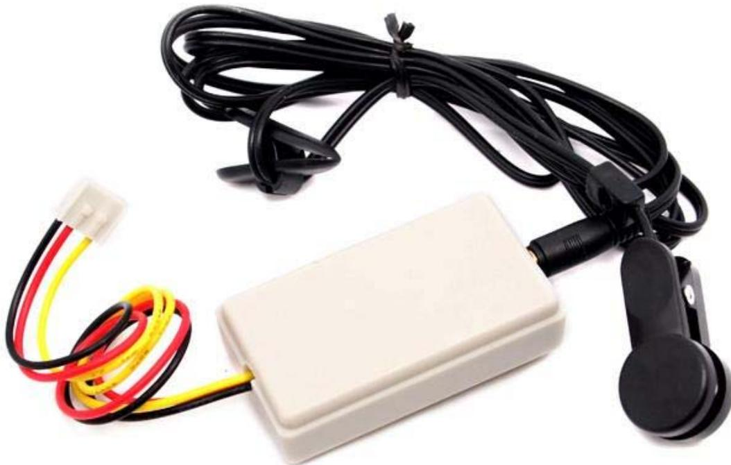
The Heart Rate Ear clip kit contains a ear clip and a receiver module. The heart rate measure kit can be used to monitor heart rate of patient and athlete. The result can be displayed on a screen via the serial port and can be saved for analysis. The entire system is a high sensitivity, low power consumption and portable.
