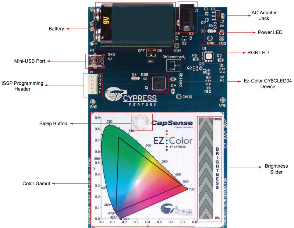
Note: For optimum performance, place the board horizontally on a flat surface.
