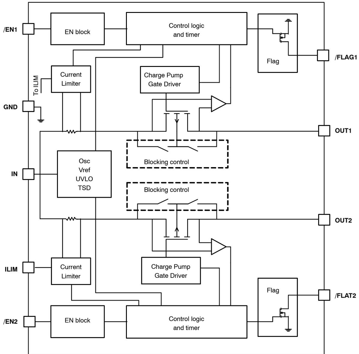
Figure 2. Block Diagram
