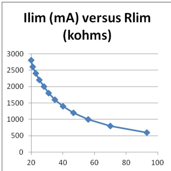
Figure 7. Typical Ilim Curve vs Rlim External Resistor
