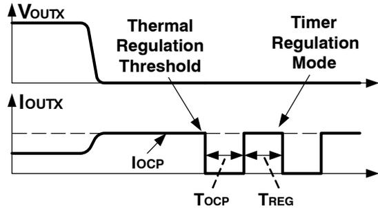
Figure 6. Short Circuit
