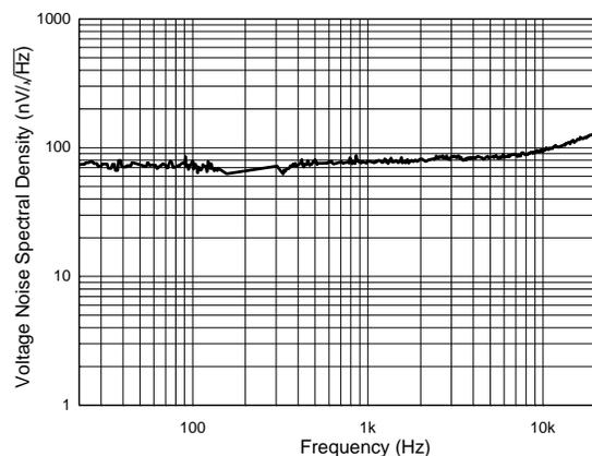
**Figure 2. Input Voltage Noise in Zero-Drift Amplifier (AS2333)**
