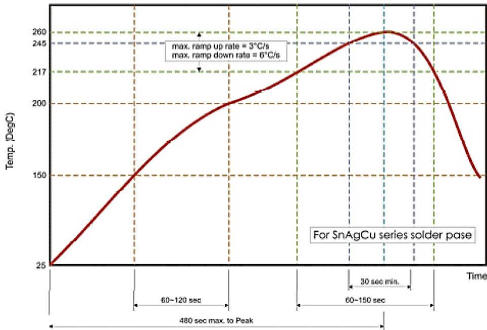
Fig 2. Infrared soldering profile for Chip Resistors
