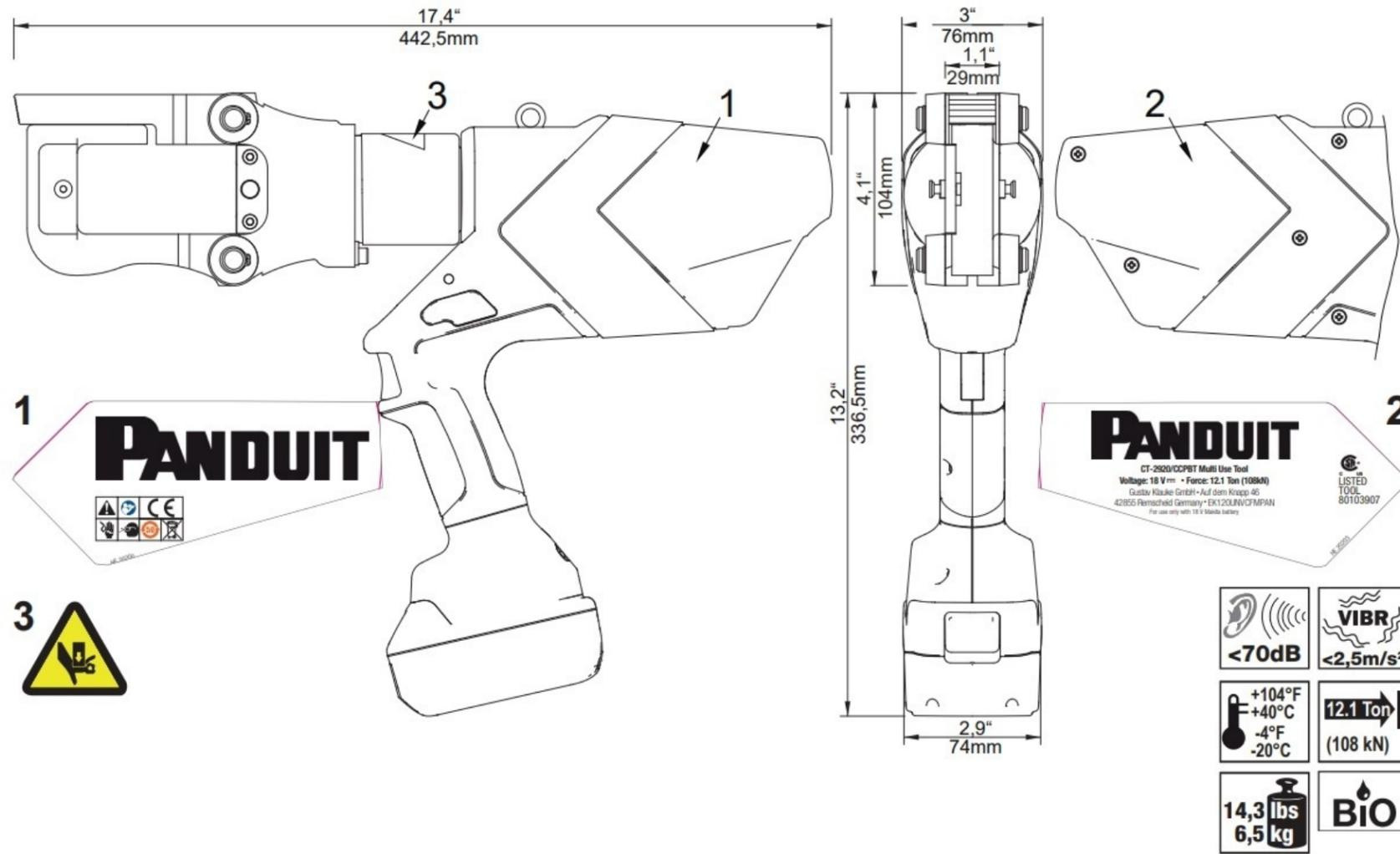
CT-2920/CCPBT, 12 TON MULTI-USE (CRIMP-CUT-PUNCH) TOOL
