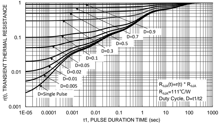
Figure 25. Transient Thermal Resistance
