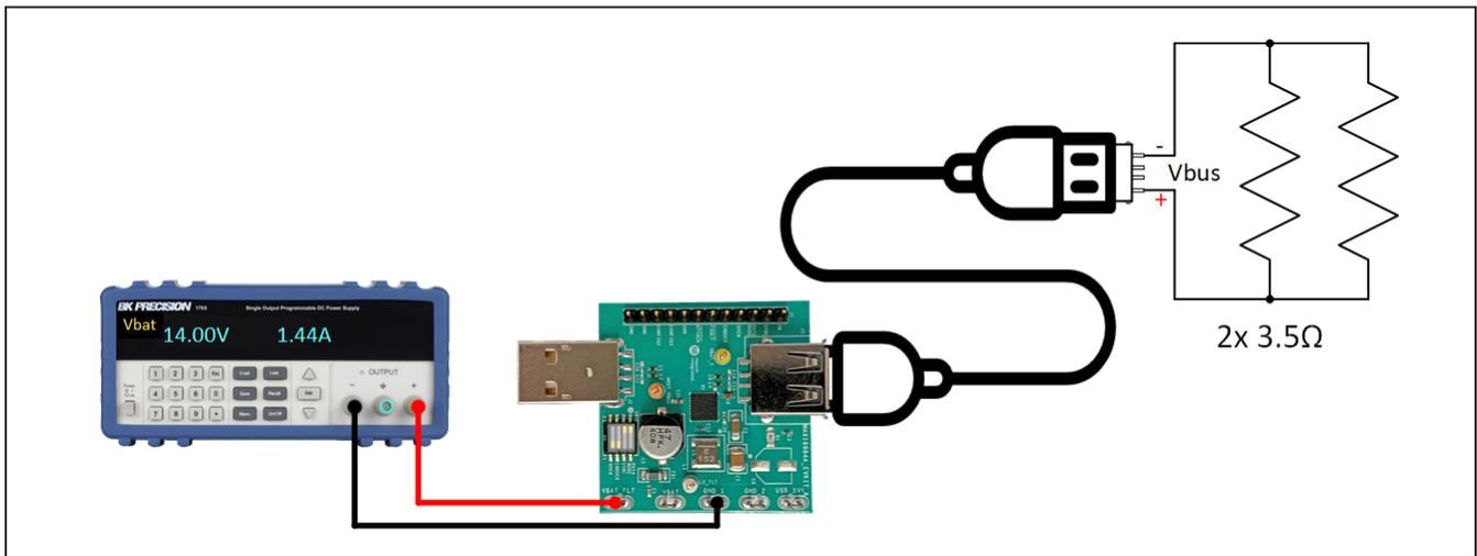
Figure 3: EV Kit Setup for Cable Compensation
