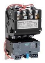
Non-reversing motor starter Size 1 Three phase full voltage Solid-state overload relay OLRelay amp range 10-40a 380-440/440-480V 50/60HZ coil Combination type No enclosure
