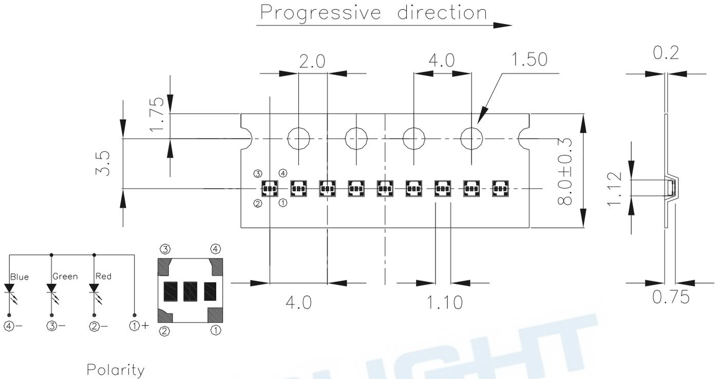
Note: Tolerances unless mentioned  $\pm 0.1$ mm. Unit = mm
